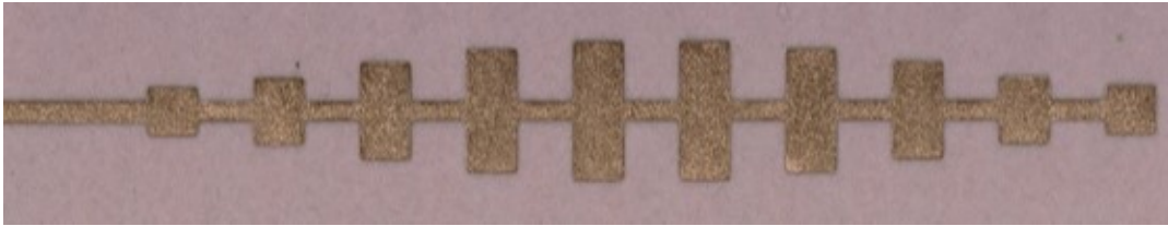
Figure 3.18: Patch antenna array with 0.5 \lambda_g spacing as viewed under the microscope with 200x zoom.
