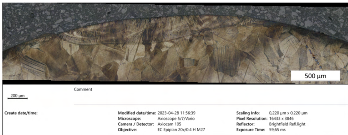
Figure D.2: Microstructure of Mn13_V2 XVI
