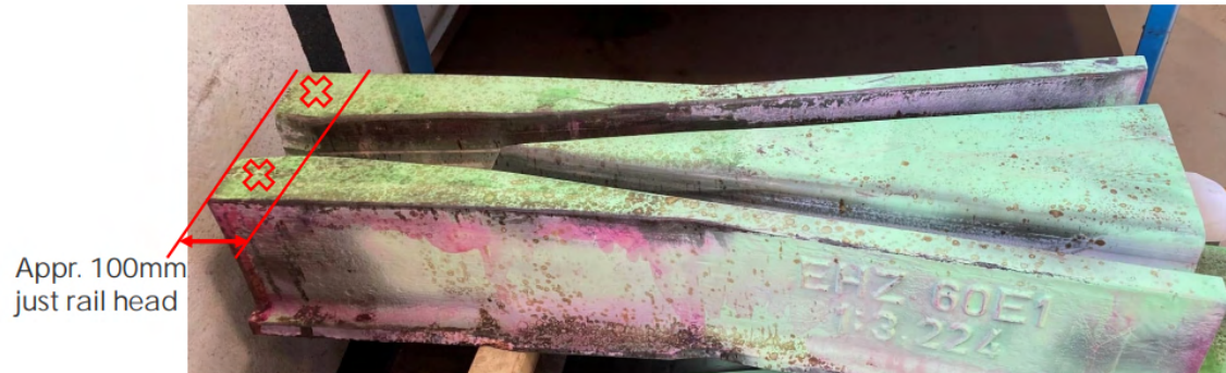
Figure 3.1: D (2017); field sample of a damaged turnout.
