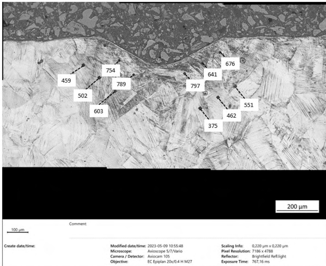
Figure 4.14: Optical microscope image of Mn13_M 2 with microhardness indents visible, specified in HV [0.1]
