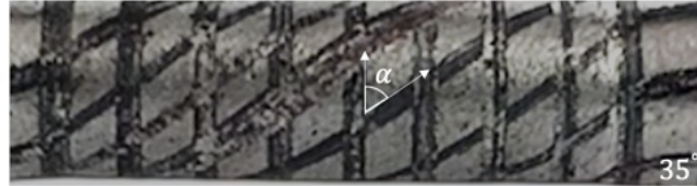
Figure 3.6: Measurement of surface shear strain, angle \alpha is measured and used to calculate \gamma , which represent surface shear strain
