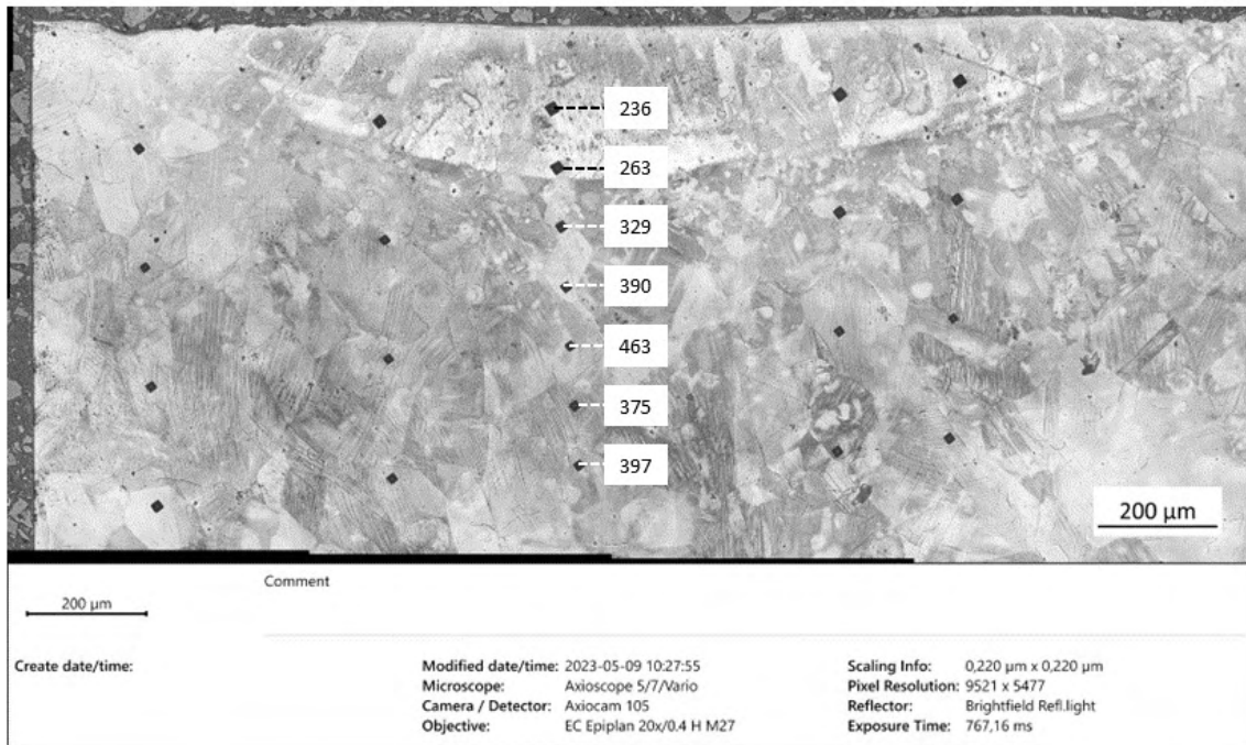
Figure 4.4: Optical microscope image of Mn13_T 4 with microhardness indents visible, specified in HV [0.1]
