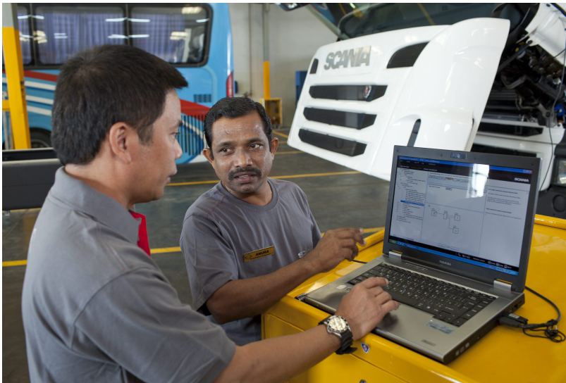
Figure 13: The picture shows an ongoing diagnostic session where the PC is connected to the truck (Scania Image Archive, property of Scania CV AB (publ)).
