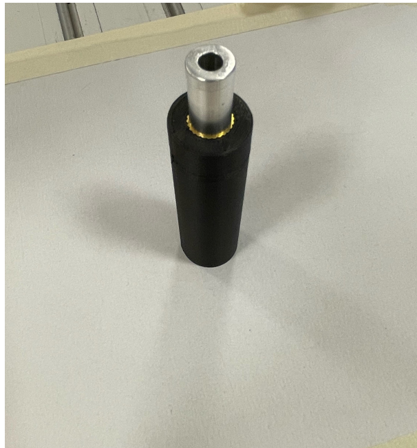
Figure 4.7: Extended nozzle to enable picking of body rivet.
