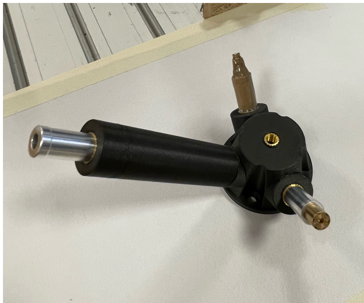
Figure 4.8: Extended nozzle mounted on the multi-nozzle holder.
