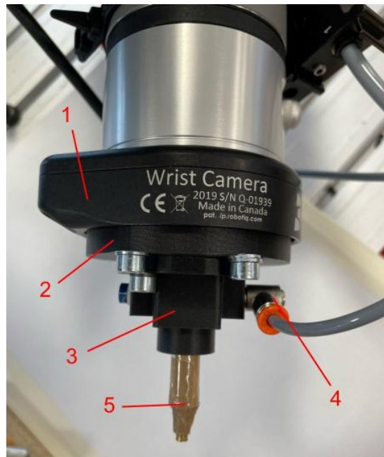
Figure 4.10: Setup of the experiment. 1: Robotiq Wrist camera, 2: Middle plate, 3: Nozzle holder, 4: Vacuum inlet, 5: Nozzle.
