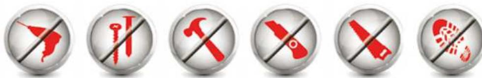
Figure 3.11 Warning labels designed for the va-Q-tec VIP (va-Q-tec 2013)
