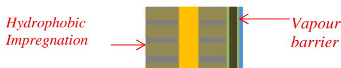
Figure 5.9 Localisation of the vapour barrier and the hydrophobic impregnation for the Alternative 2
