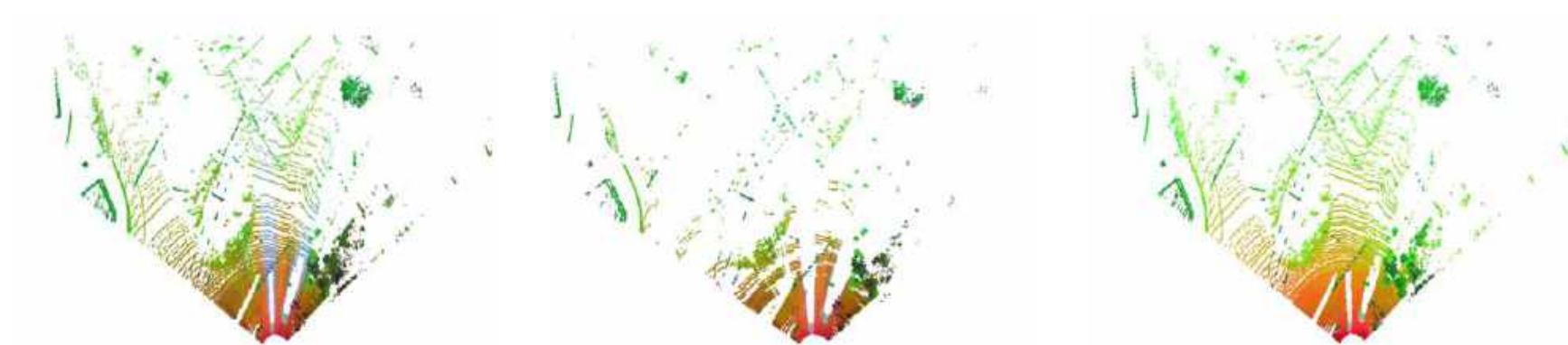
(a) Feature cloud with bleeding issue. Car features (in blue) are leaking behind the cars.
