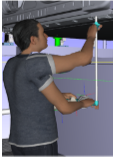
Figure 7. Operator not using spindle to tighten screws (Volvo cars, 2023)
