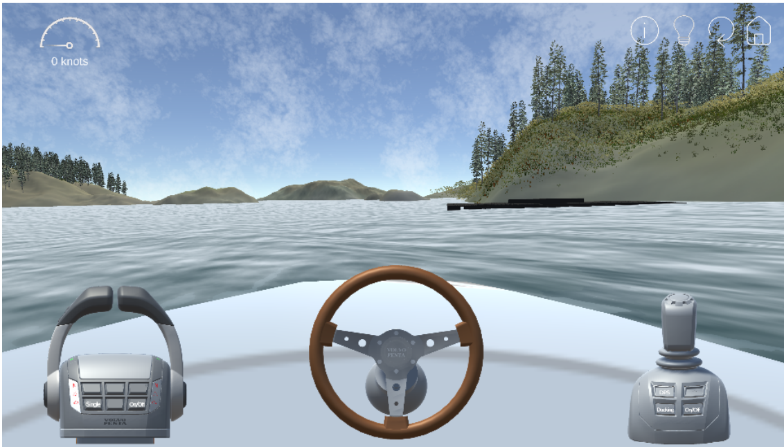
Figure 7.16: The view from inside the cockpit, including a Volvo Penta Dual lever/Throttle, Steering wheel and Joystick
