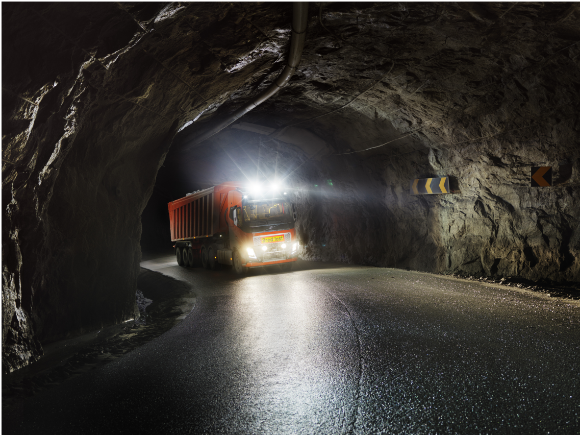
Figure 4.1: Autonomous Volvo truck driving in one of the tunnels.[27]
