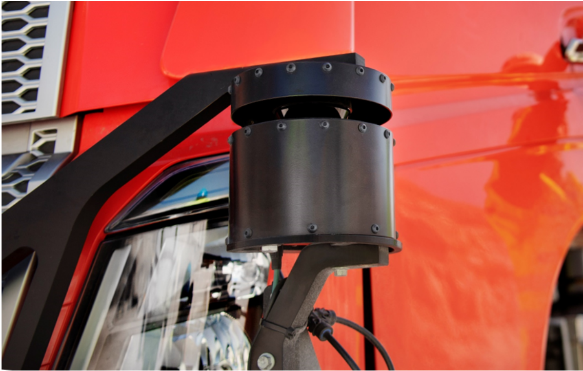
Figure 4.3: Current LiDAR helmet installed in the project. The picture is cropped.[32]
