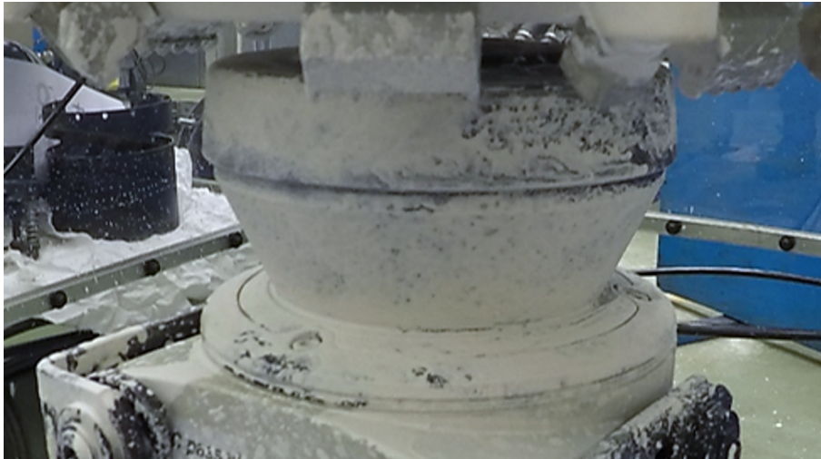
Figure 7.7: Hardened wet mix applied to the LiDAR.
