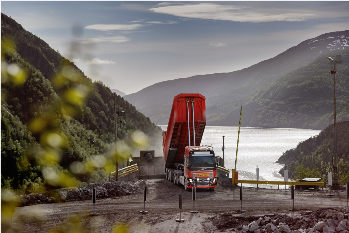
Figure 4.2: Autonomous Volvo truck offloading at the crusher.[28]
