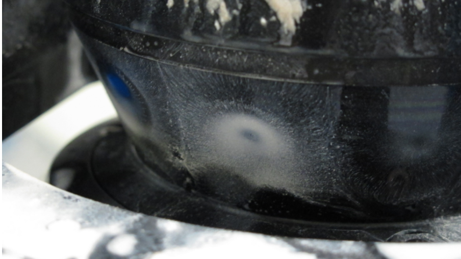
Figure 7.14: Re-appearance of dirt developed on the optics cover where the air stream is directed from the current cleaning system.
