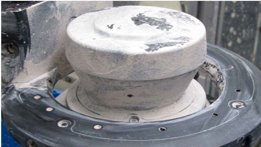
Figure 7.13: Hardened wet mix applied to the LiDAR prior to testing the current cleaning system.
