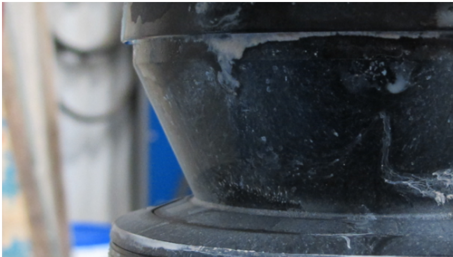
Figure 7.9: Re-appearance of dirt on the optics cover and shelf
