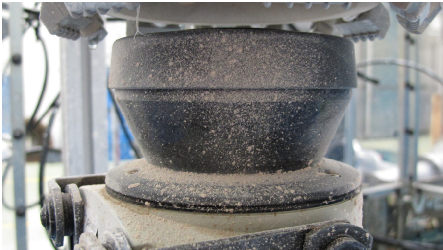
Figure 7.12: Dust mix applied to the LiDAR.
