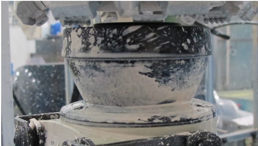
Figure 7.10: Wet mix applied to the LiDAR.
