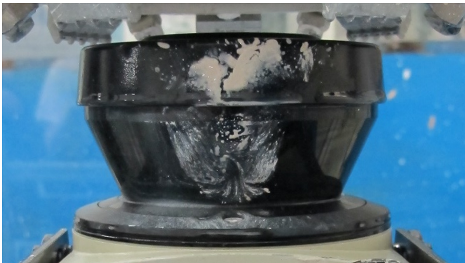
Figure 7.8: Neglected area of the LiDAR after applying water and air with Divided Prototype.
