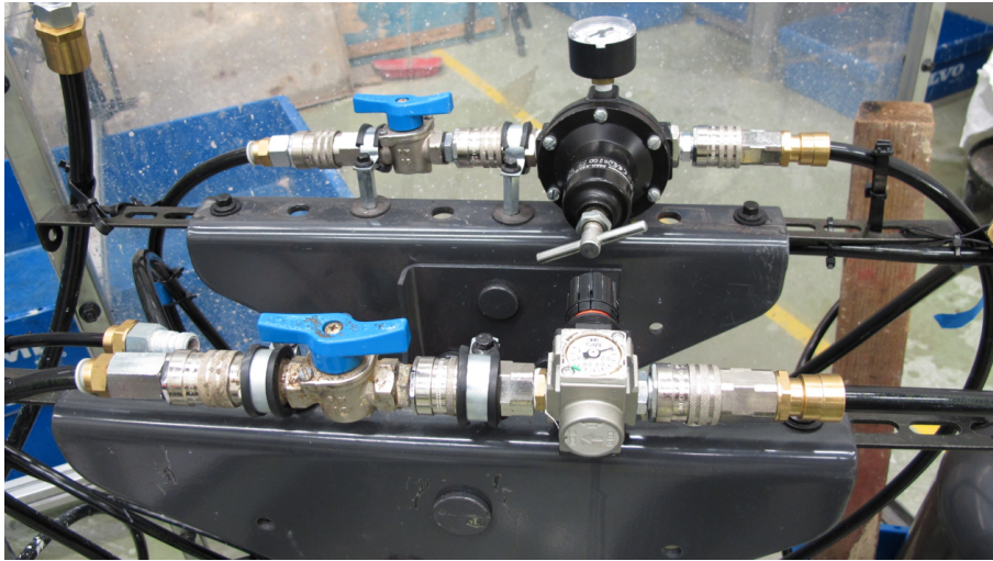
Figure 7.3: The regulators used during the testing.
