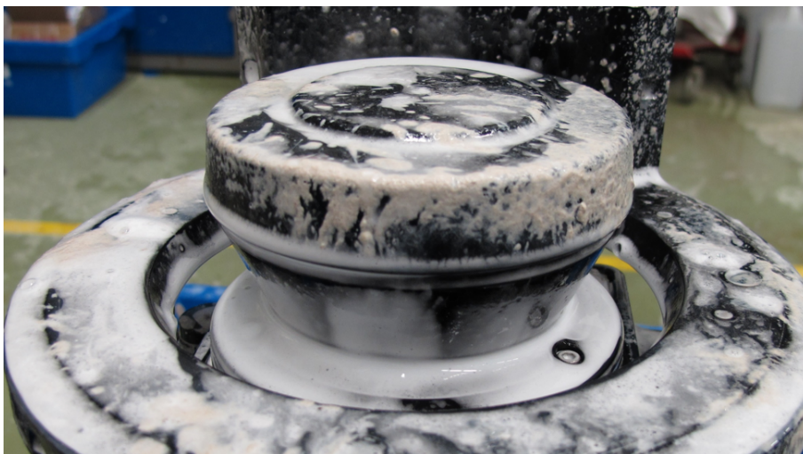
Figure 7.15: The foam on the LiDAR after applying air for 8 seconds with the current cleaning system.
