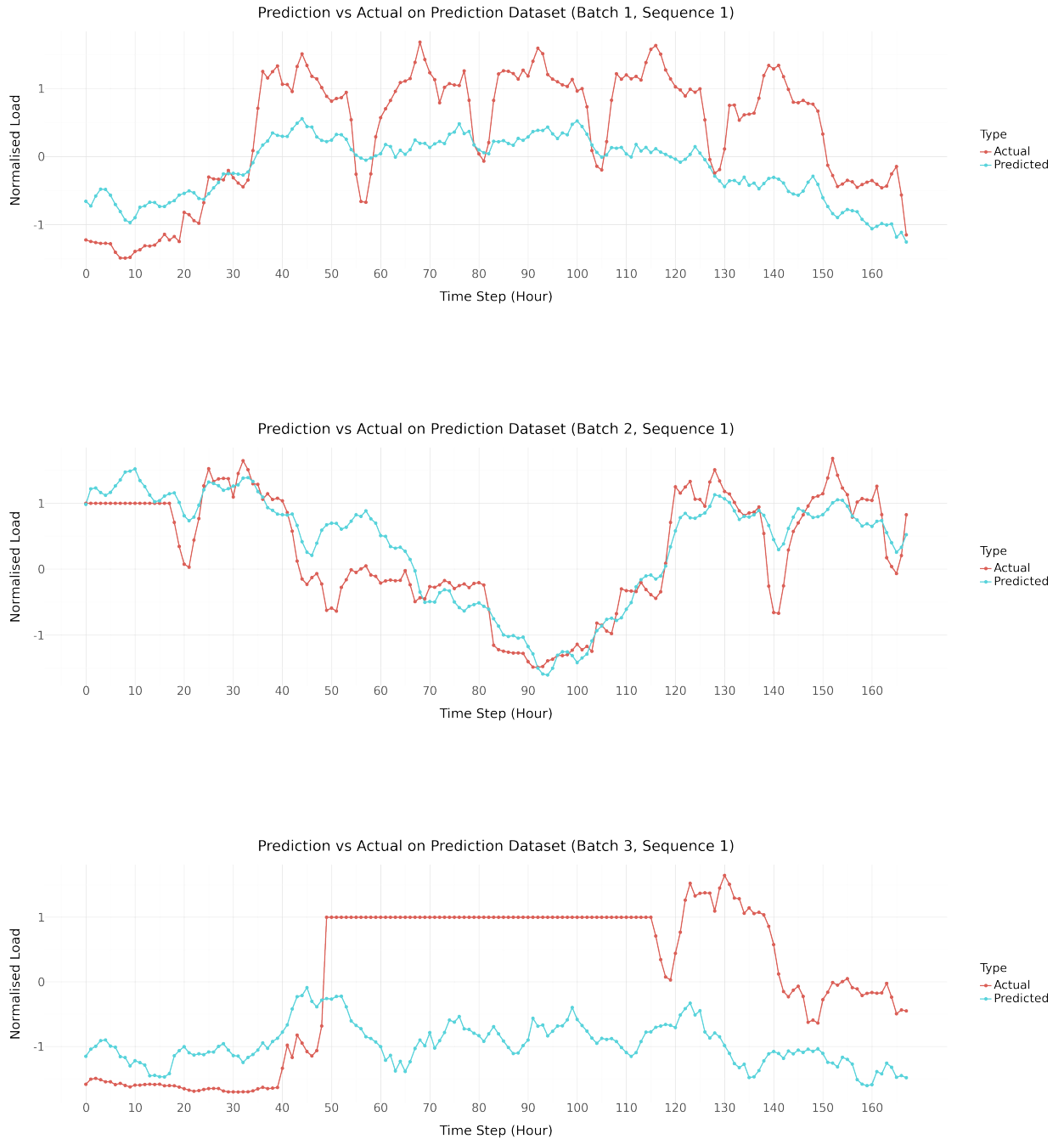
Figure A.6: Bidirectional LSTM: Prediction vs Actual on Prediction Dataset for three different batches.
