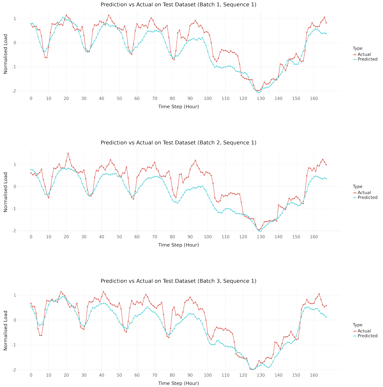
Figure A.1: Vanilla LSTM: Prediction vs Actual on Test Dataset for three different batches.
