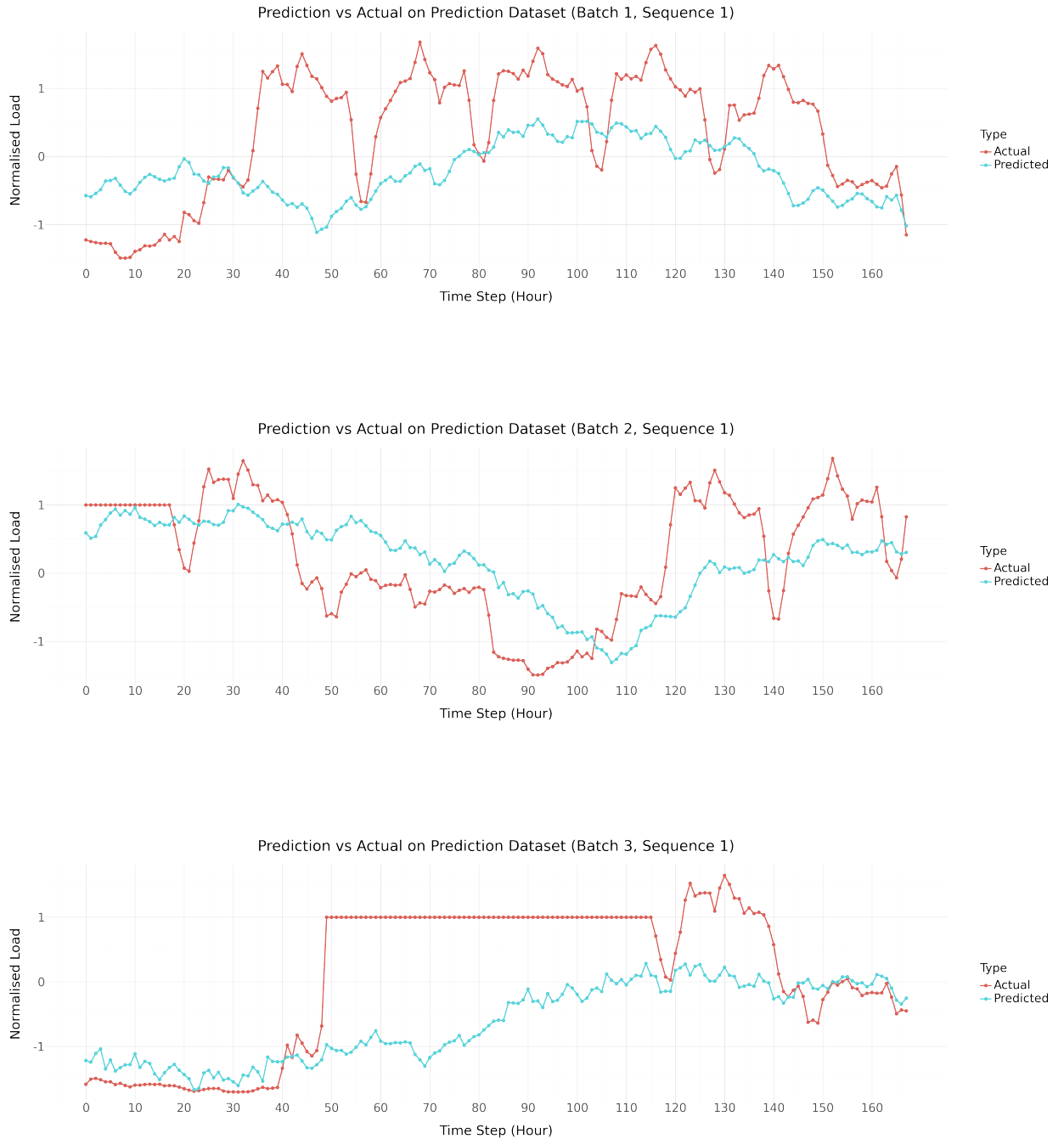
Figure A.4: Stacked LSTM: Prediction vs Actual on Prediction Dataset for three different batches.
