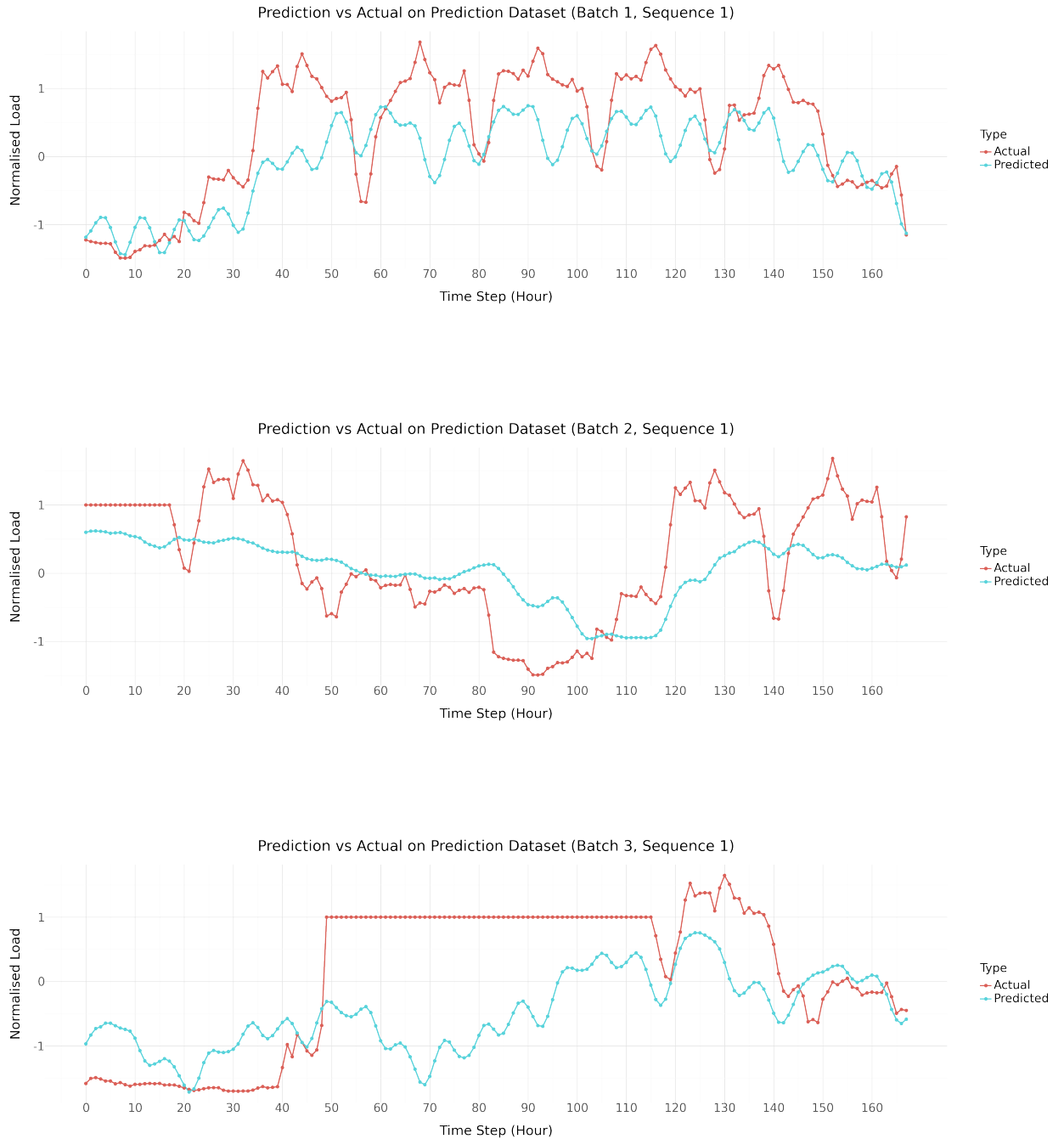
Figure A.8: CNN-LSTM: Prediction vs Actual on Prediction Dataset for three different batches.
