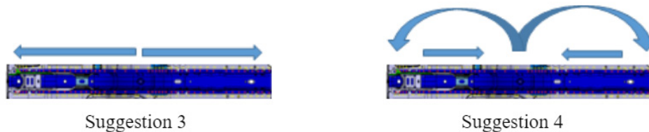
Figure 31: The difference in the welding direction for suggestion 3&4
