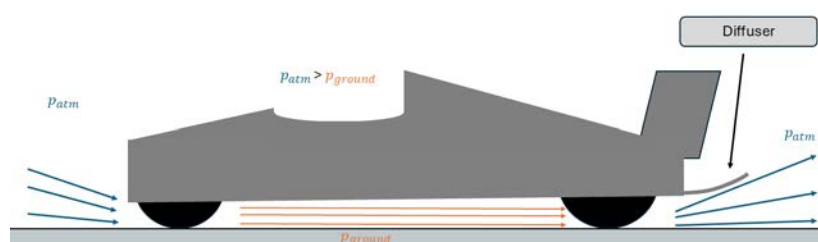
Figure 2.10: 2D illustration of the venturi effect of a race car with a diffuser.
