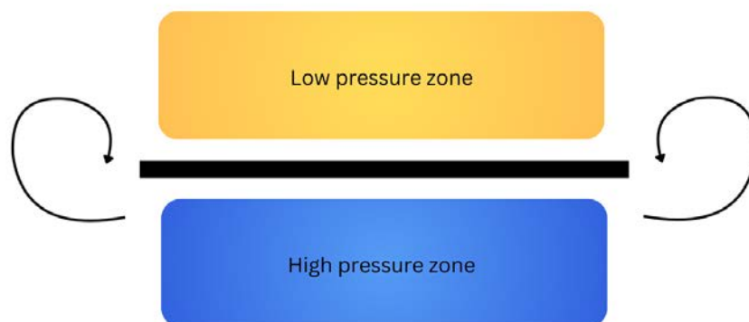
Figure 2.5: Graphic representation of end tip vortex
