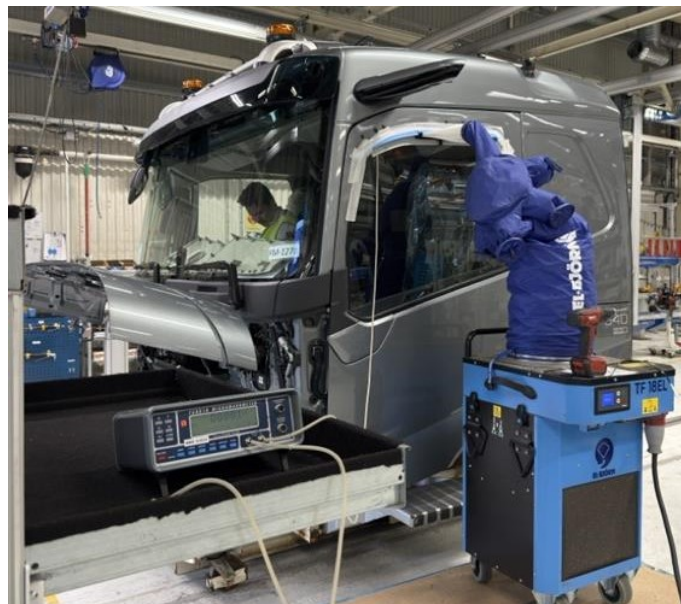
Figure 3.3: Main test setup used for pressurization and experimentation.
