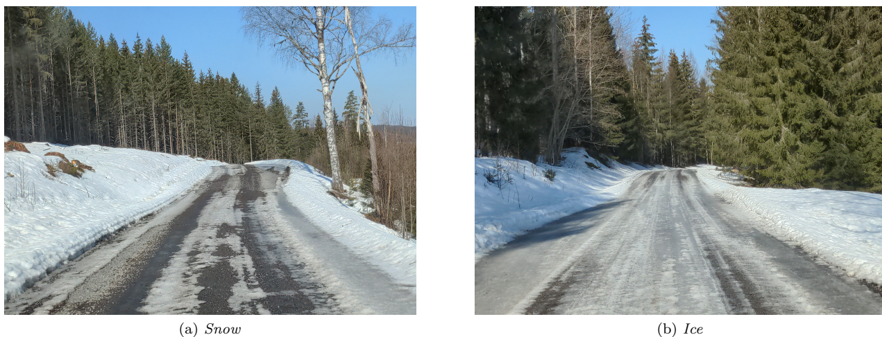
Figure 6.3.1: Illustration of the subjective distinction between snow- and ice-covered roads.
