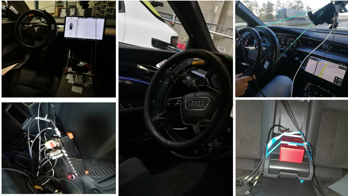
Figure 3.4: Competitor car measurement set-up, including steering effort sensor, IMU, Dewesoft DEWE 43 and Logitech HD Pro C920
