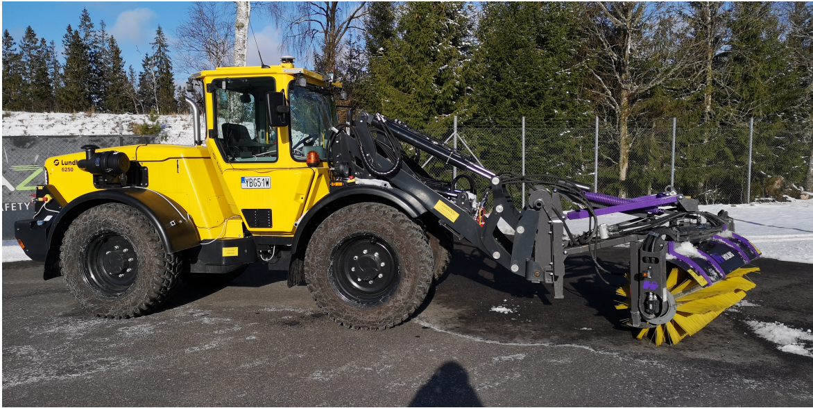
Figure 2.1: Picture of the maintenance vehicle. On the roof of the cab, the mounted GNSS unit can be seen as a white disk.
