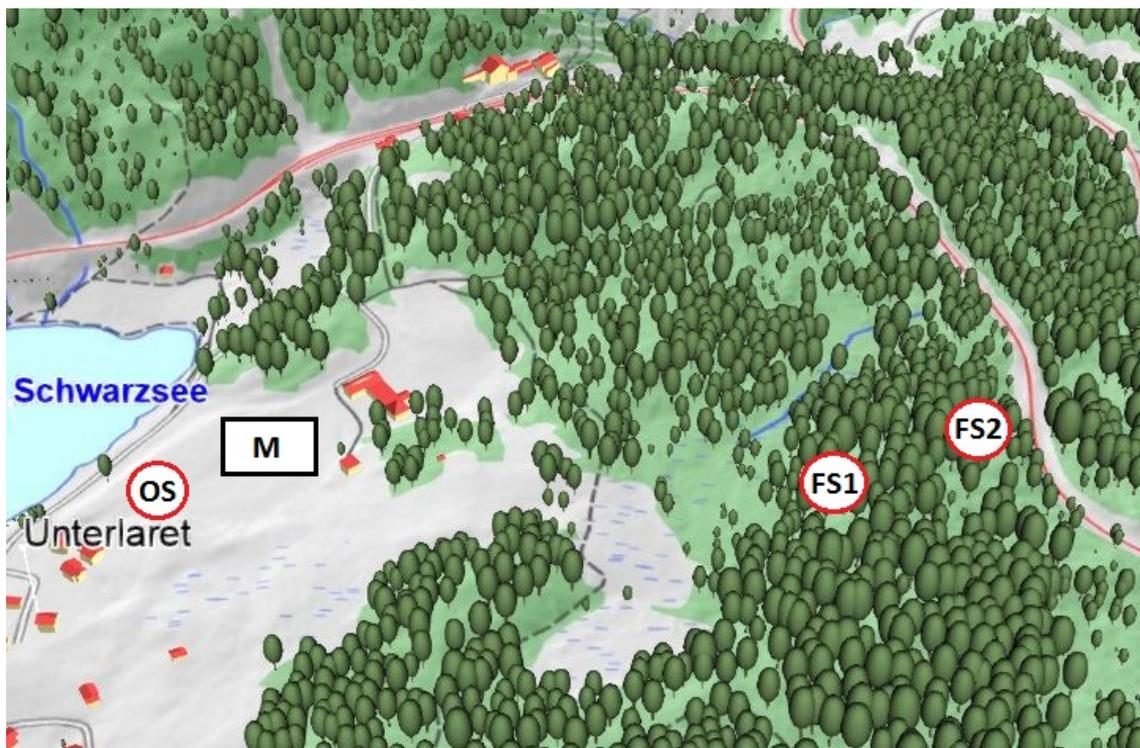
**Figure 3.2:** The three circles represent the three station sites, Open Site (OS), Forest site 1 FS1 and Forest site 2 FS2. The new permanent meteorological station in Laret is marked with a capital M. This station only started operations in the 2019 season. The map is generated with the online map tool from The Swiss Federal Geographical Information Geodata © swisstopo [17].
