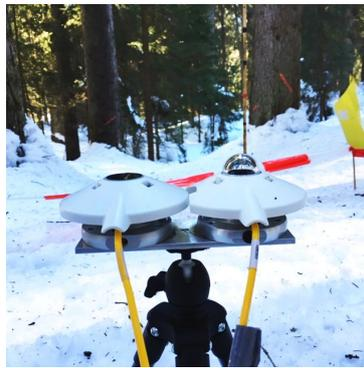
**Figure 3.8:** Side-view of SWR and LWR sensors
