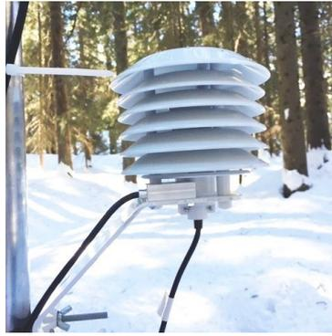
**Figure 3.5:** Air temperature Sensor
