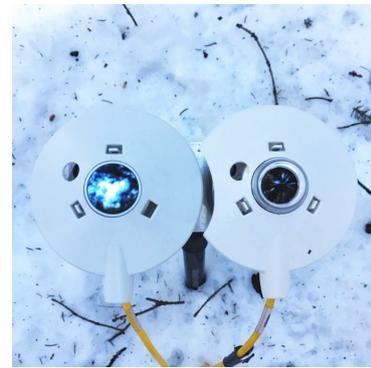
**Figure 3.9:** Top view of SWR, LWR sensors
