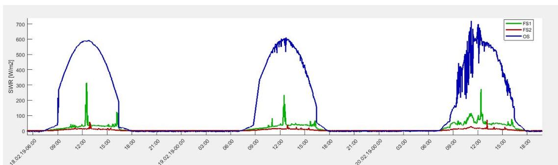
**Figure 3.11:** Observed non-aggregated data of SWR during a 3 day period, with 2 consecutive days of clear skies followed by a day of overcast.
