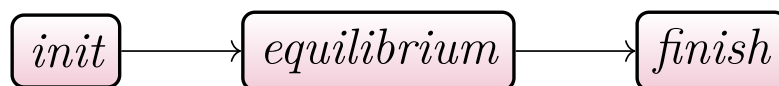
Figure 3.1: Simple workflow illustration consisting of three actors. The first initiates the plasma scenario, the second calculates the plasma equilibrium and the third saves data and closes the simulation correctly. The arrows represent the direction of information flow.
