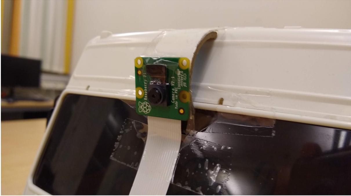
Figure 10: Raspberry PI-camera V2
