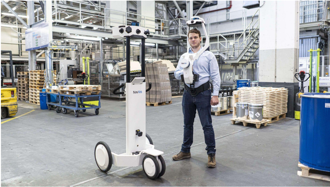
Figure 2.1: A person standing next to NavVis' 3D scanning equipment
