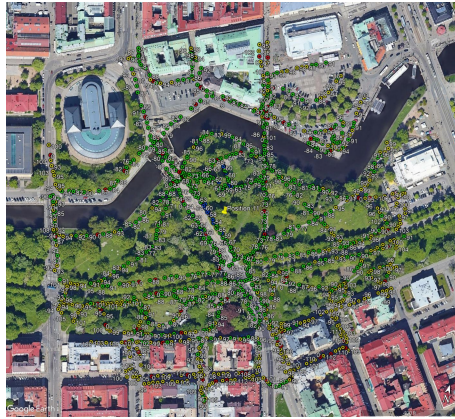
Figure 4.11: Area testing data points for position 11 with a base station in an open setting
