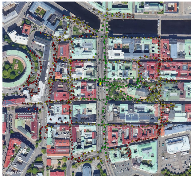
Figure 5.1: RSSI values spatial weighted averaging in SF 9 area test: base station position 1
