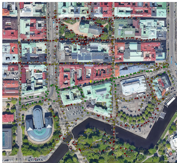
Figure 5.2: RSSI values spatial weighted averaging in SF 9 area test: base station position 6
