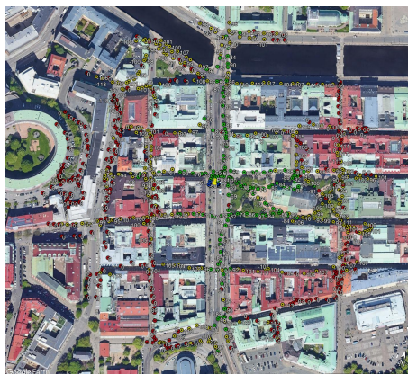
Figure 4.10: Area testing data points for position 1 with base station in a semi-open setting
