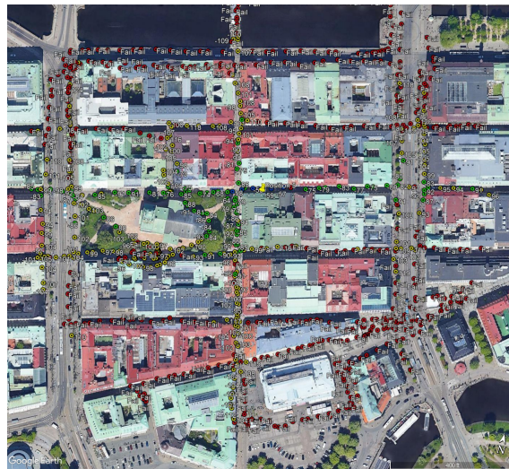
Figure 4.12: Area testing data points for position 5 with a base station in an alley/closed setting
