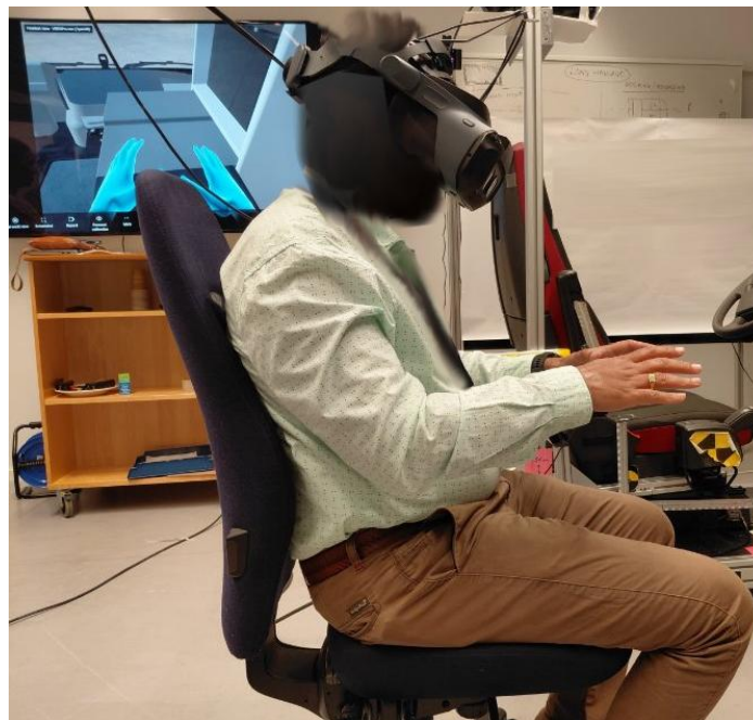
Figure 58. Expert evaluating ergonomic aspects of the cab concept in the VR environment.
