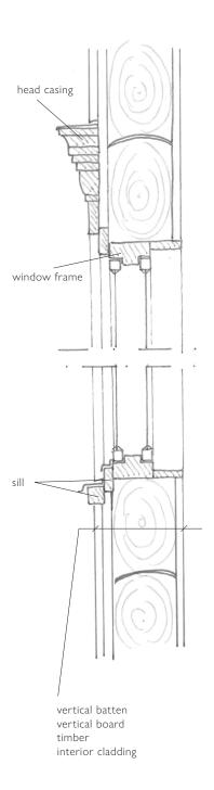
Figure 45. Detail sketch of the window.
