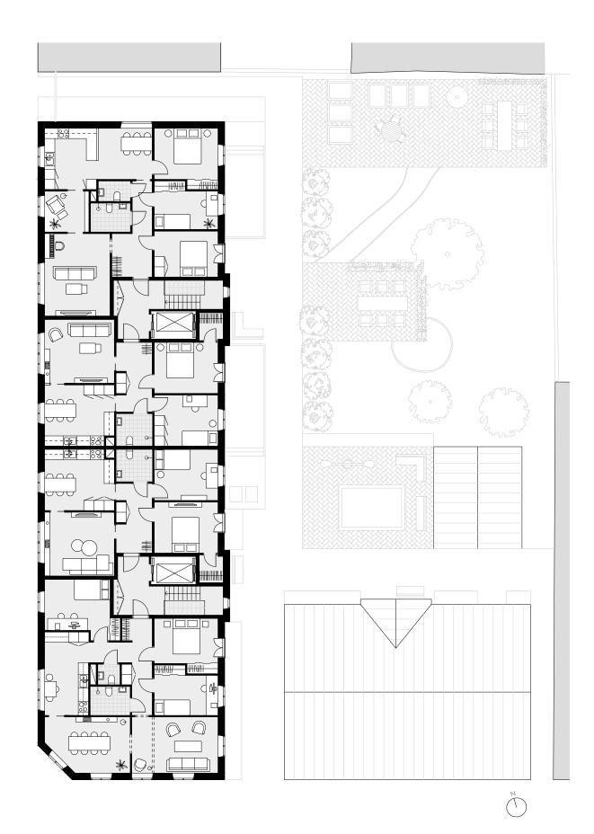
Figure 83. Third floor, scale 1:200.
