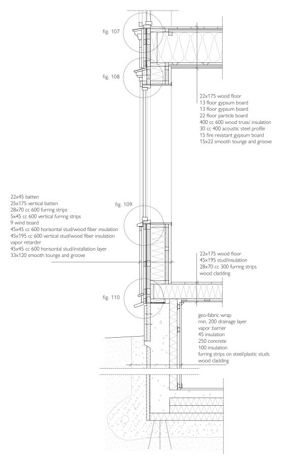
Figure 105. Section detail part 1, scale 1:25.
