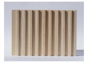
Figure 14. Board and batten.
