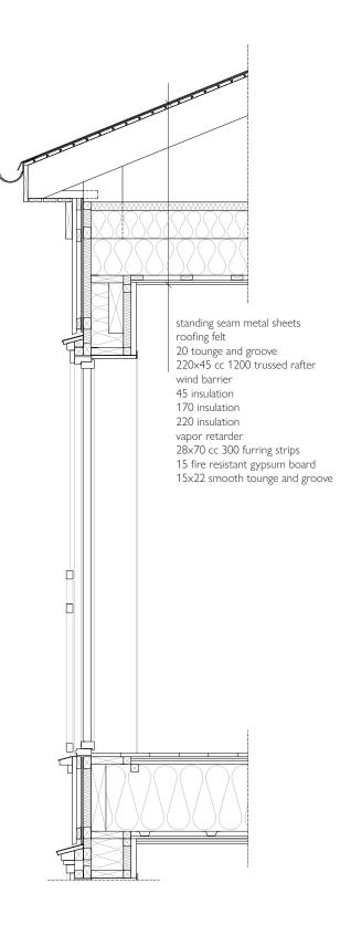
Figure 101. Section detail part 2, scale 1:25.
