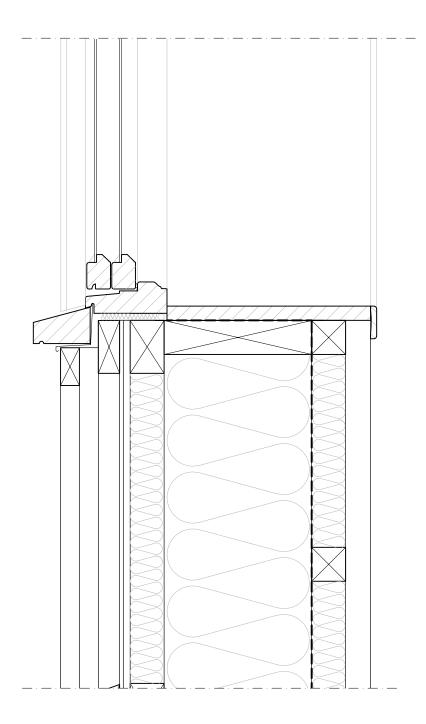
Figure 109. Detail showing window and sill, scale 1:5.
