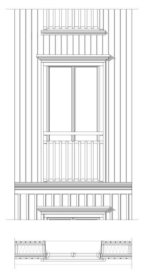
Figure 104. French balcony detail, scale 1:25.
