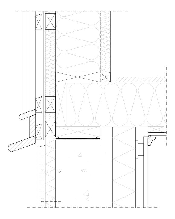
Figure 110. Detail showing wall meeting foundation, scale 1:5.
