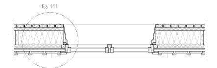
Figure 106. Window detail, scale 1:25.
