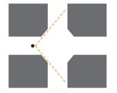
Figure 35. Sightlines with chamfered corners.
