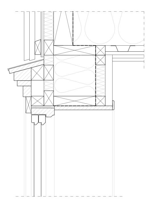
Figure 108. Detail showing window and head casing, scale 1:5.
