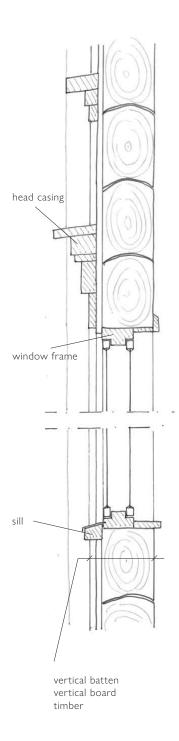
*Figure 55.* Detail sketch of the window on the first floor.
