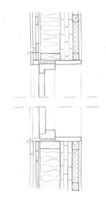
Figure 20. Principle of a CLT wall.
