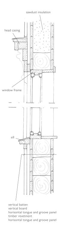
Figure 48. Detail sketch of the window
