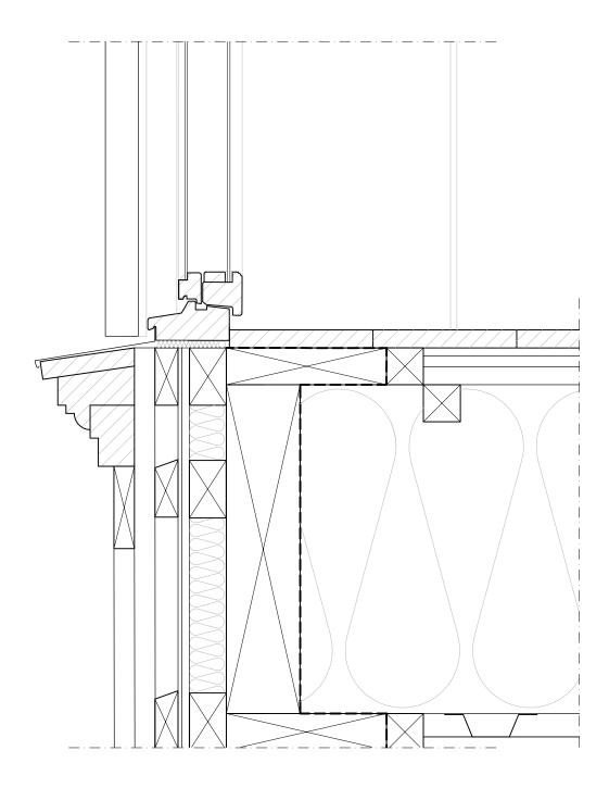
Figure 107. Detail showing french balcony, scale 1:5.
