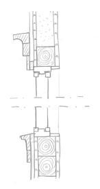
*Figure 17.* Principle of a timber wall.
