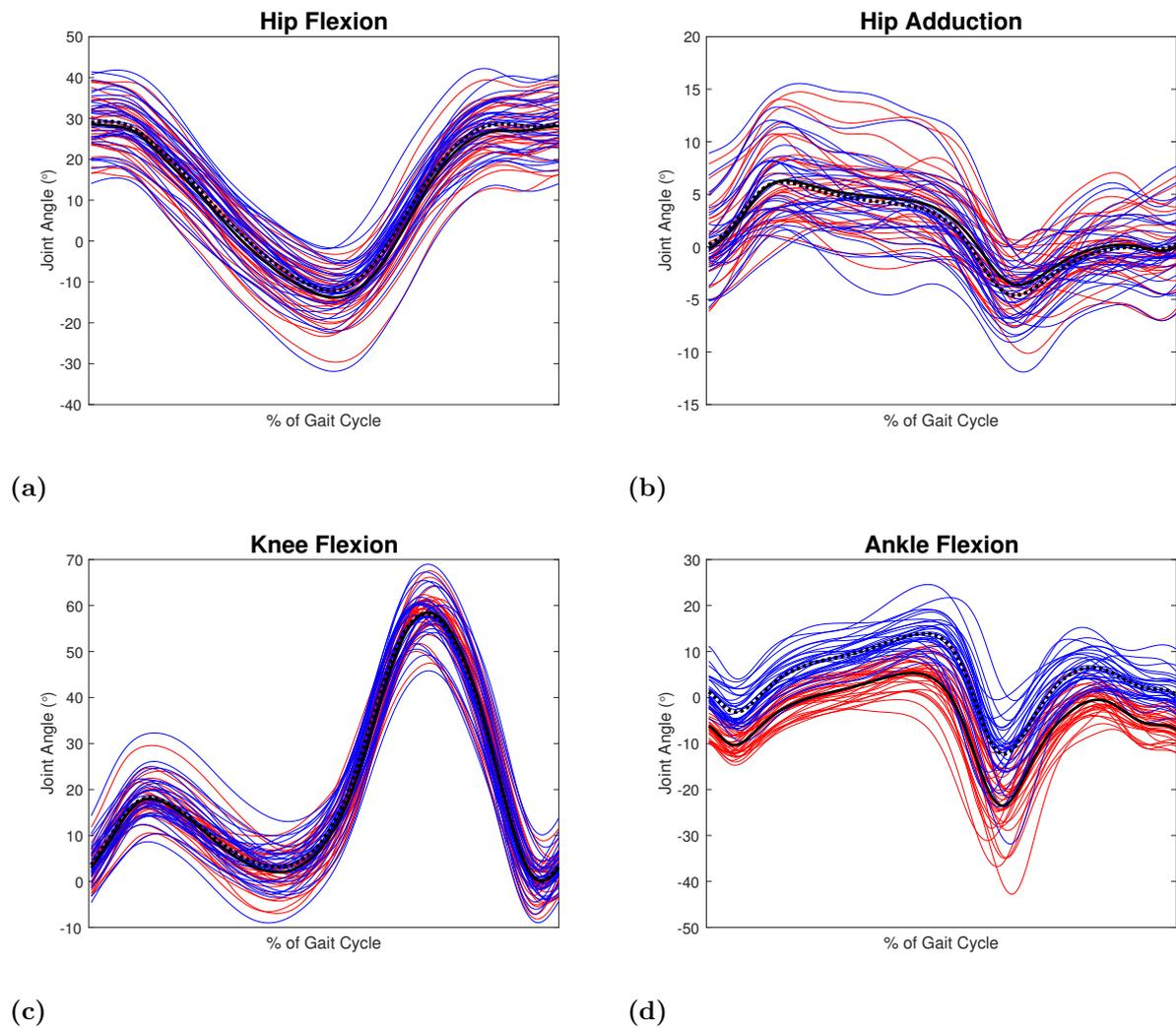
**Figure A.1:** Plots of the analysed angles. Figure a) shows hip flexion, b) hip adduction, c) knee flexion, d) ankle flexion. The red lines represent the IOR model with dashed line as the mean, the blue lines represent the Lundberg model with full line as the mean.
