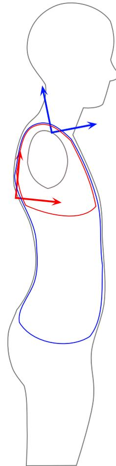
**Figure 5.1:** The trunk and thorax segments and their respective coordinate system. The Lundberg trunk segment in blue and the IOR thorax segment in red.
