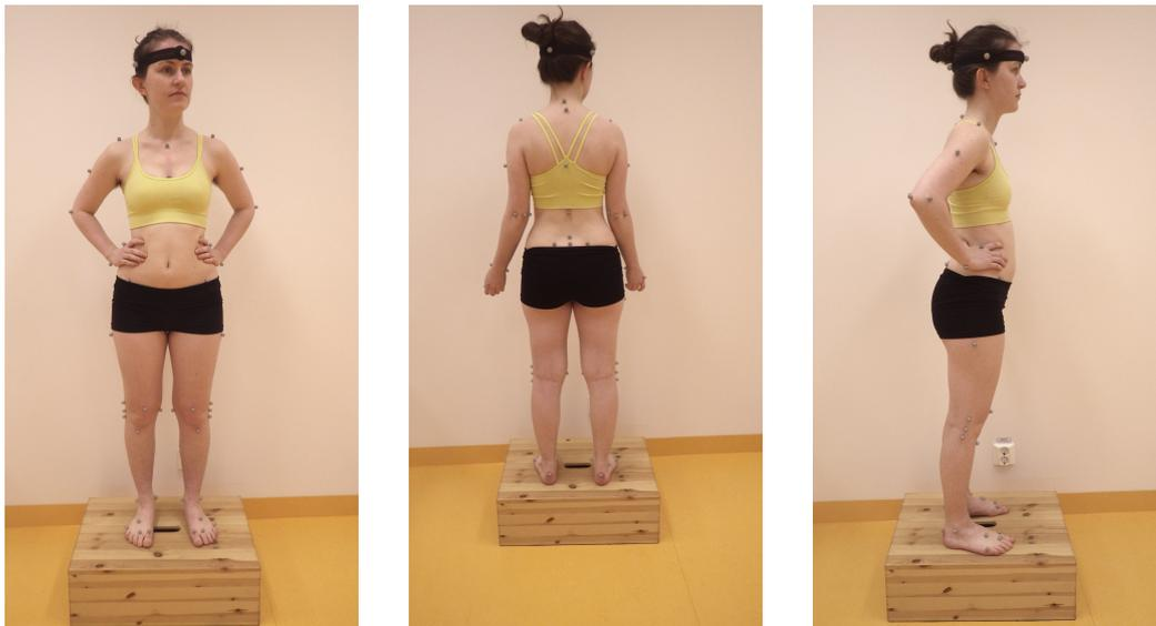
**Figure 3.2:** The marker placement on subject with the hybrid skin marker model.
