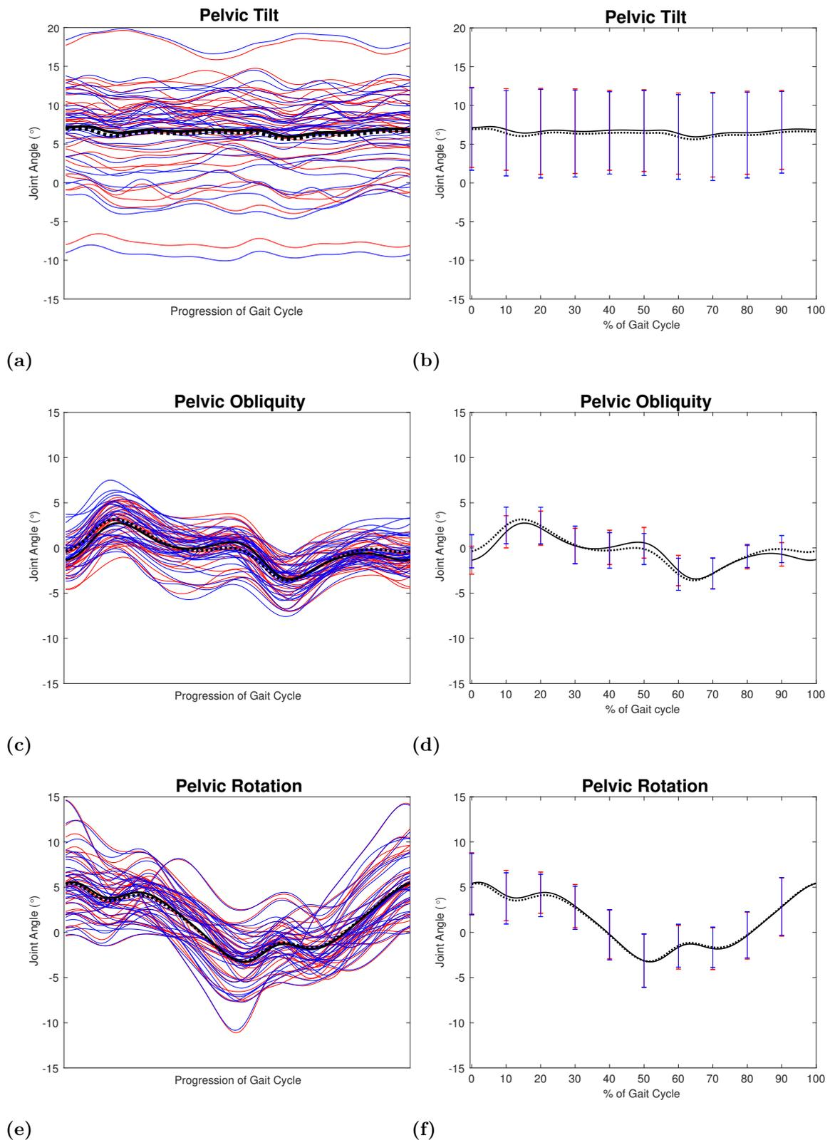
**Figure 4.1:** Figure a, c and e show plots for pelvic angles with subject means (red for IOR and blue for Lundberg) and model mean (solid line for IOR and dotted line for Lundberg). Figure b, d and f show plots for model mean with  $\pm 1$  st.dev. at the 10 chosen points. The standard deviation were calculated using the subject means at the chosen points. Statistically significant points are denoted with \*.
