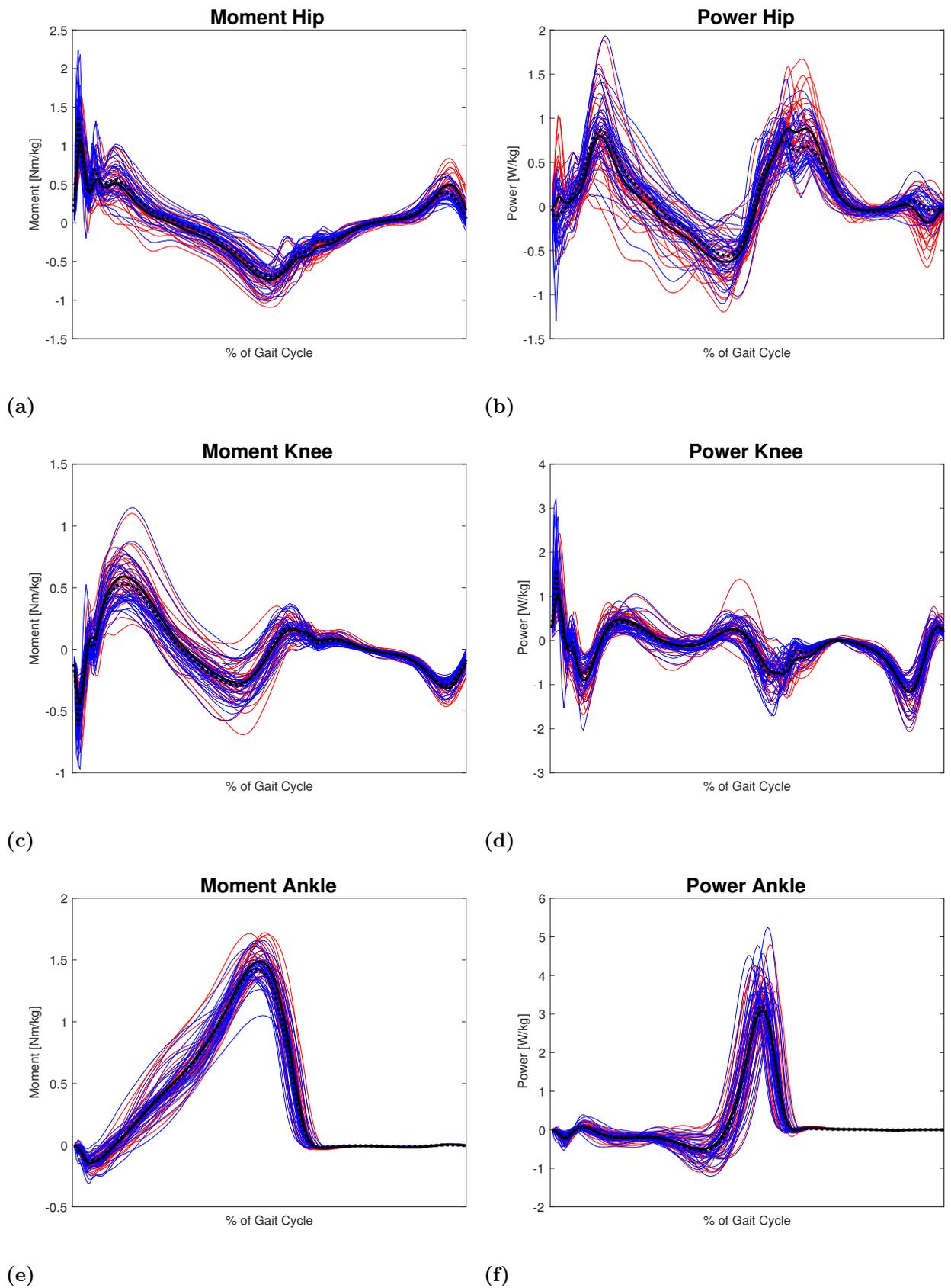
**Figure A.2:** The plots of moment and power for some joints. Figure a) shows hip moment, b) hip power, c) knee moment, d) knee power, e) ankle moment and f) ankle power. The red lines represent the IOR model with dashed line as the mean, the blue lines represent the Lundberg model with full line as the mean.
