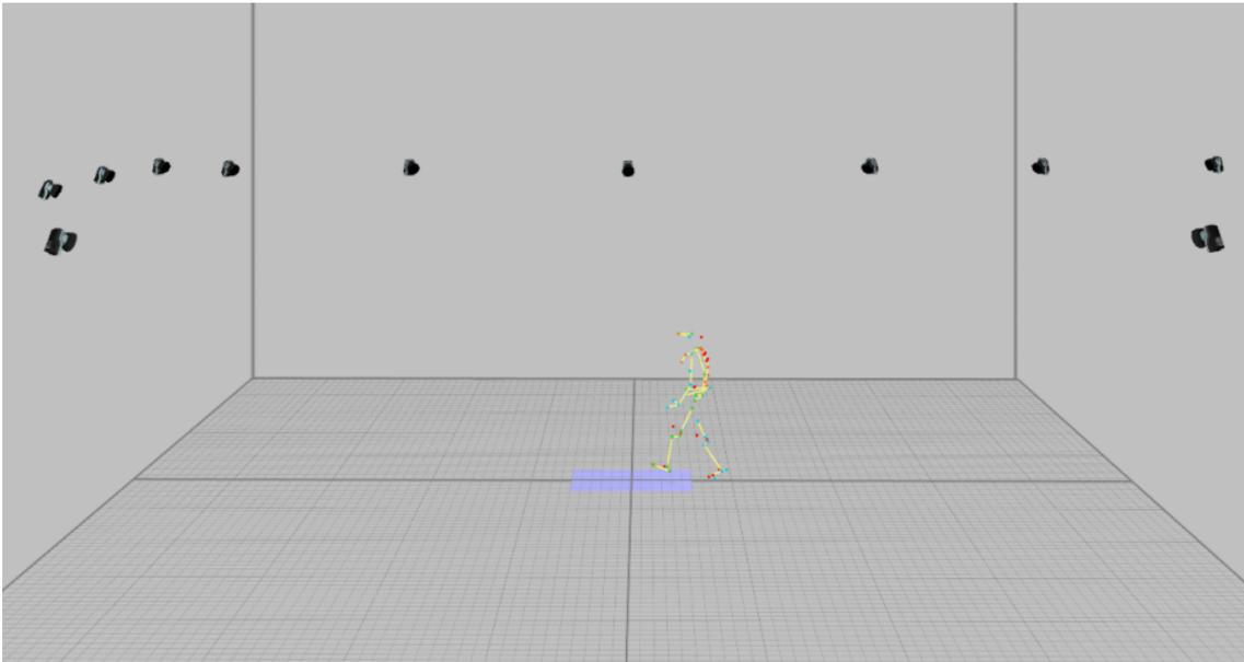
**Figure 2.1:** The measuring space with cameras mounted on the walls and four force plates sunken into the floor
