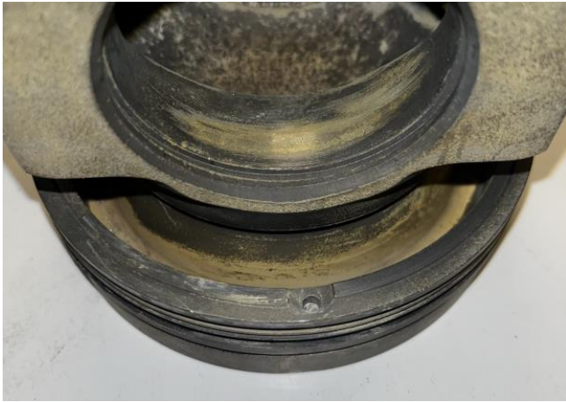
Figure E10.1. Piston 10 cooling gallery after cleaning.
