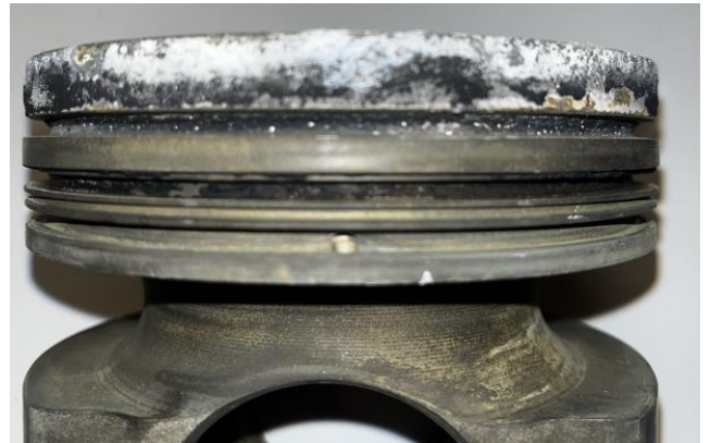
Figure E4.2. Piston 4 upper compression groove after cleaning.
