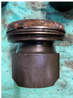
Figure 4. Excessive corrosion on Top Land.
