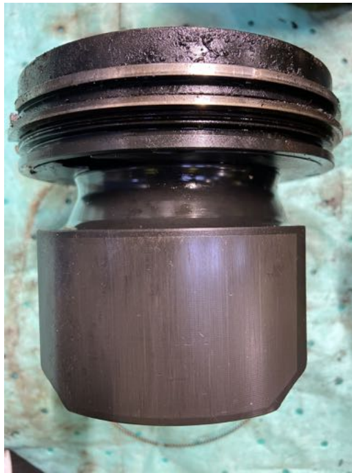
(b) Side view, some visible carbon build-up to top land. Acceptable wear.
