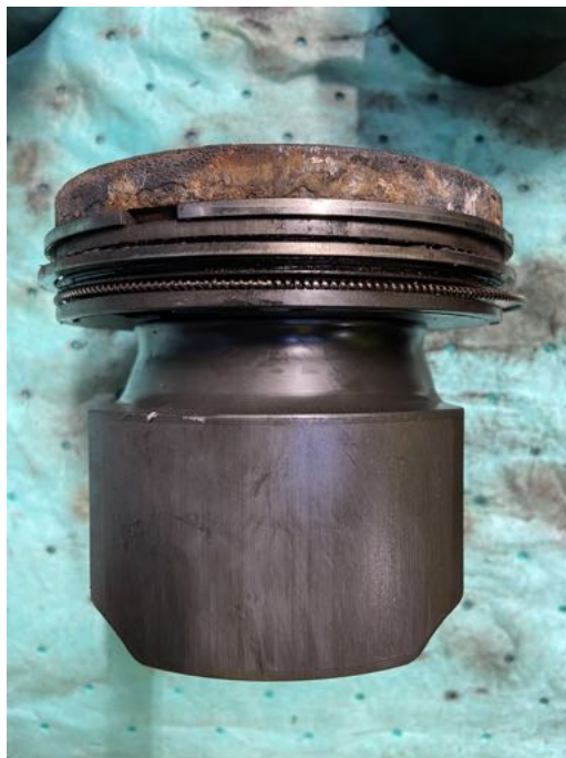
(d) Side view, significant corrosion on the top land. Not acceptable wear.
