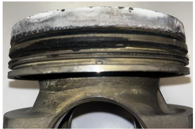
Figure E2.2. Piston 2 upper compression groove after cleaning.
