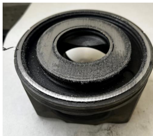
Figure E15.2. Cross sectional view of piston 15 bottom part of cooling gallery after cleaning.
