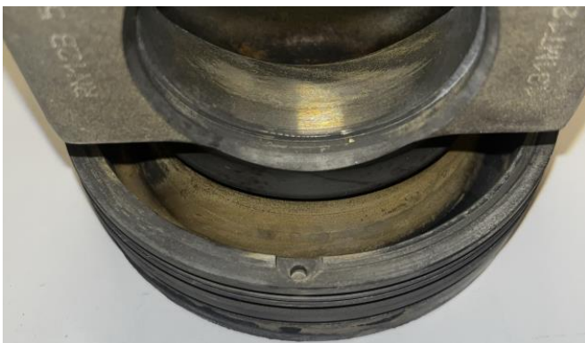
Figure E3.1. Piston 3 cooling gallery after cleaning.
