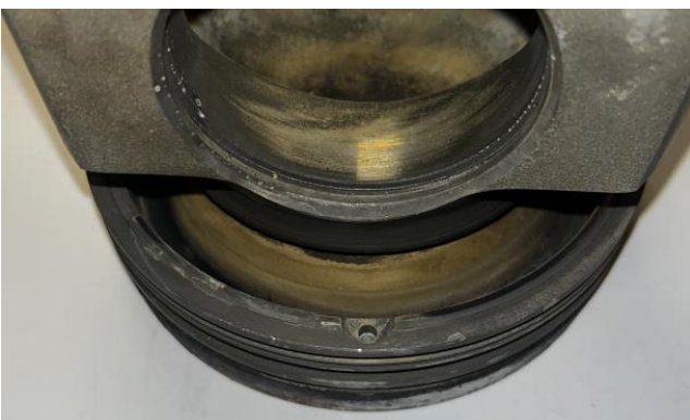
Figure E6.1. Piston 6 cooling gallery after cleaning.
