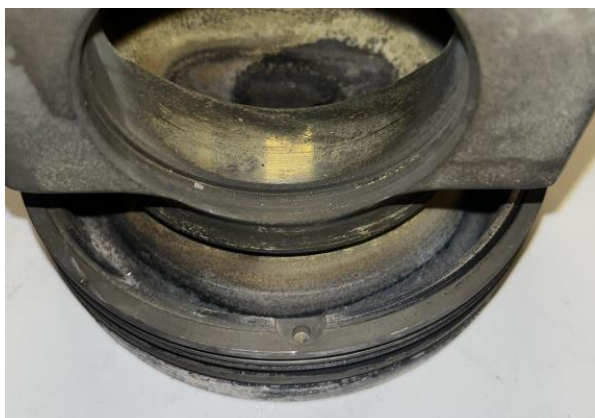
Figure E9.1. Piston 9 cooling gallery after cleaning.
