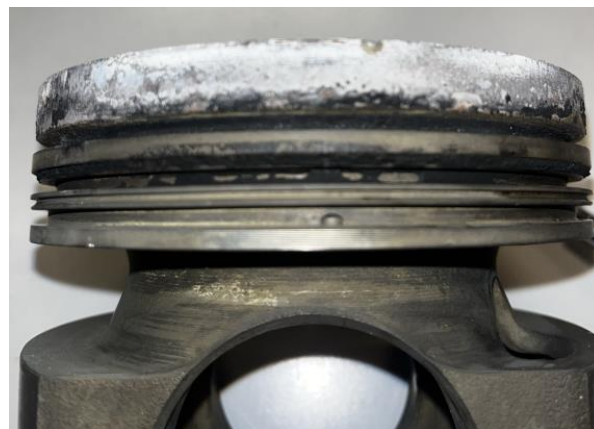
Figure E8.2. Piston 8 upper compression groove after cleaning.
