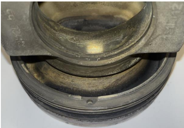
Figure E2.1. Piston 2 cooling gallery after cleaning.
