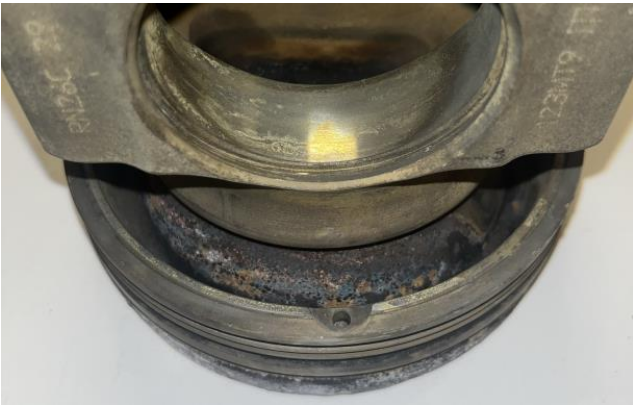
Figure E4.1. Piston 4 cooling gallery after cleaning.
