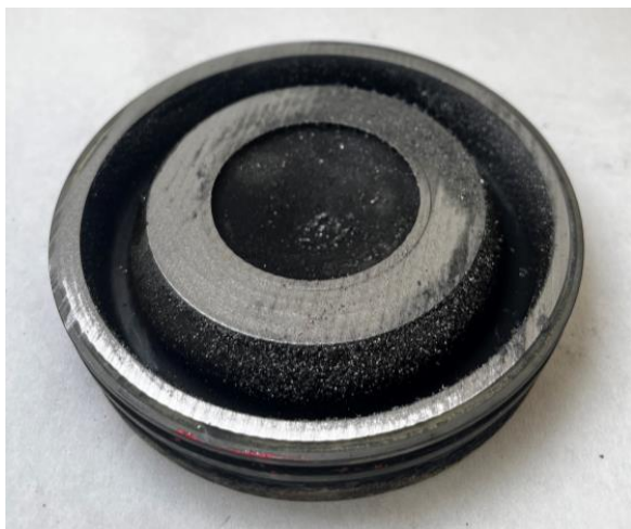
Figure E15.1. Cross sectional view of piston 15 top part of cooling gallery after cleaning.
