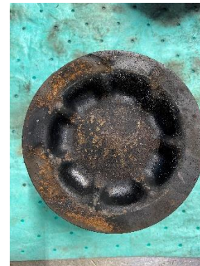
Figure 5. Excessive corrosion on Crown.
