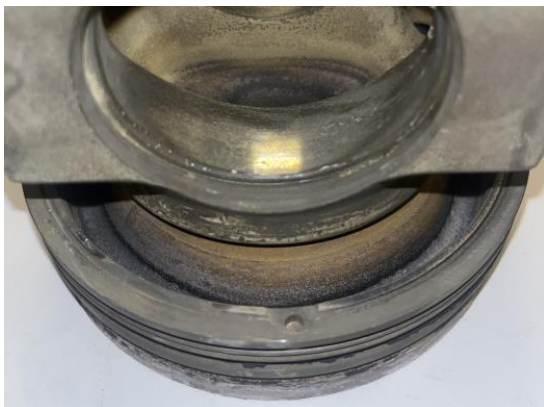
Figure E8.1. Piston 8 cooling gallery after cleaning.
