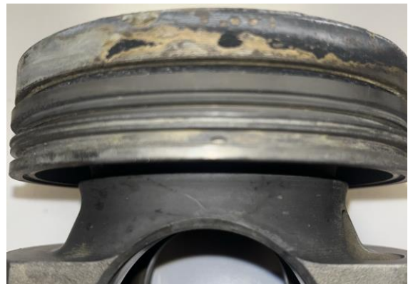
Figure E3.2. Piston 3 upper compression groove after cleaning.
