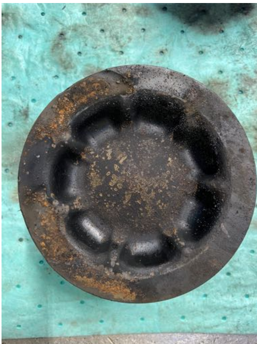
(c) Top view, significant corrosion on the bowl. Not acceptable wear.
