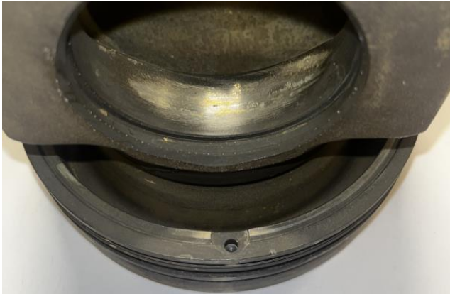
Figure E1.1. Piston 1 cooling gallery after cleaning.
