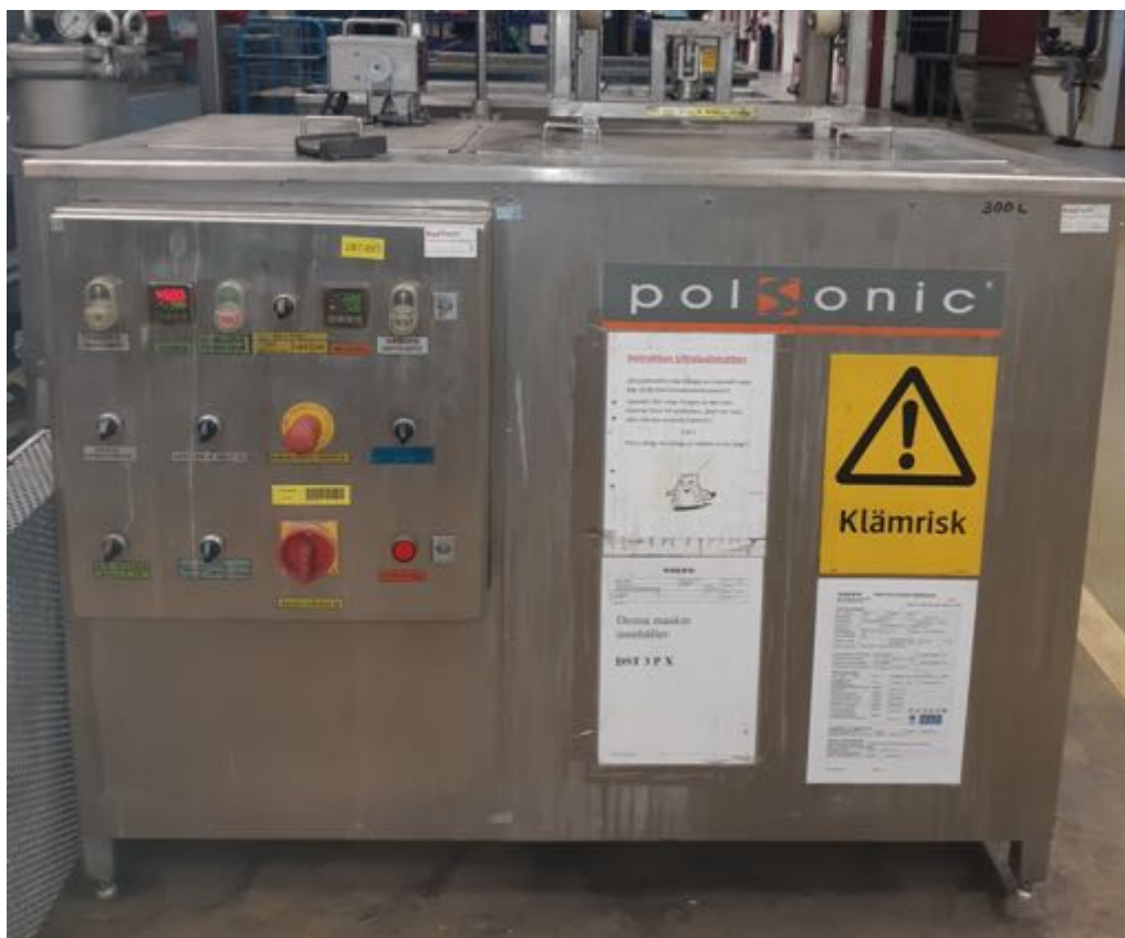
Figure 3.2: The ultrasonic cleaner, Polysonic Sonic-150, at the REMAN plant in Flen, Sweden.
