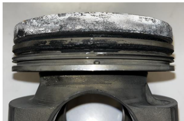
Figure E9.2. Piston 9 upper compression groove after cleaning.
