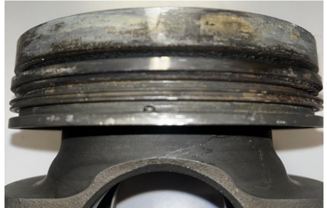
Figure E1.2. Piston 1 upper compression groove after cleaning.
