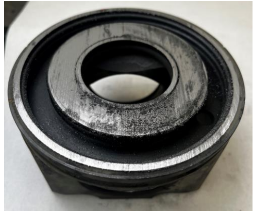
Figure E13.2. Cross sectional view of piston 13 bottom part of cooling gallery after cleaning.
