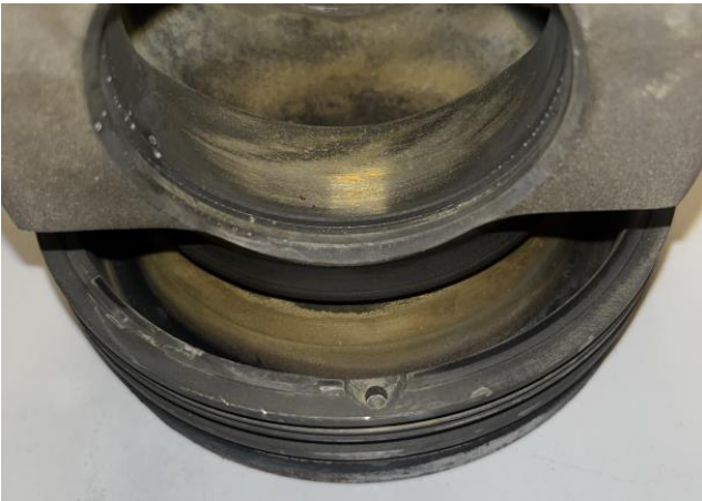
Figure E5.1. Piston 5 cooling gallery after cleaning.
