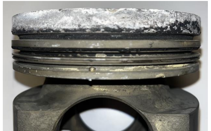
Figure E5.2. Piston 5 upper compression groove after cleaning.
