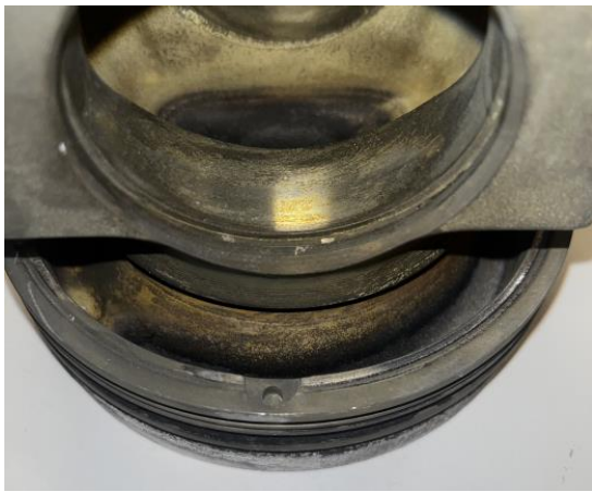
Figure E7.1. Piston 7 cooling gallery after cleaning.
