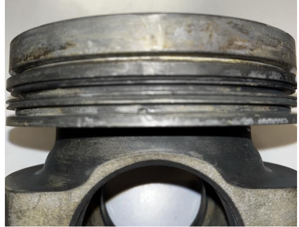
Figure E10.2. Piston 10 upper compression groove after cleaning.
