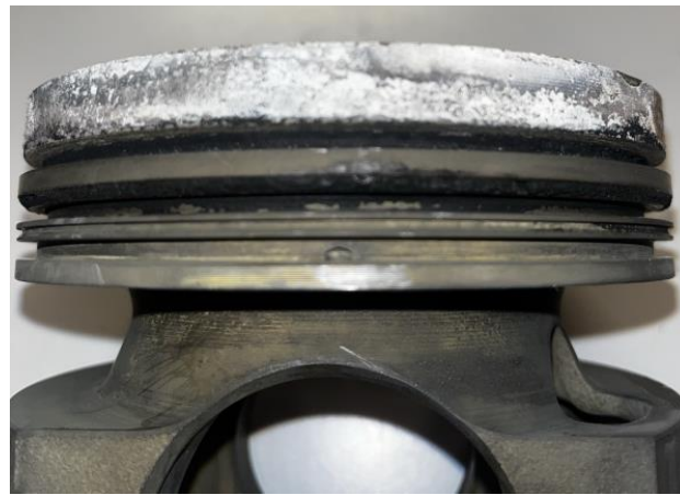
Figure E7.2. Piston 7 upper compression groove after cleaning.
