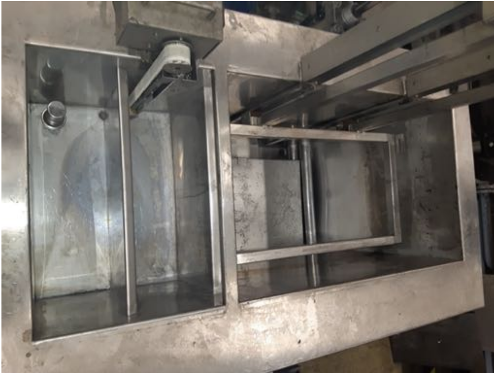
Figure 3.3: The inside of the ultrasonic cleaner, Polysonic Sonic-150, at the REMAN plant in Flen, Sweden.
