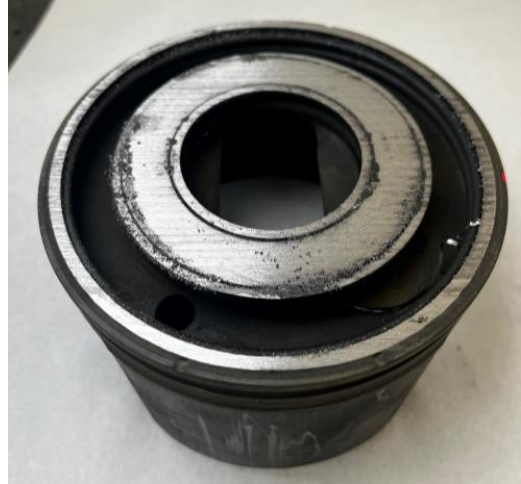
Figure E11.2. Cross sectional view of piston 11 bottom part of cooling gallery after cleaning.
