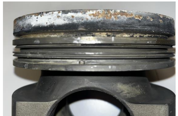
Figure E6.2. Piston 6 upper compression groove after cleaning.
