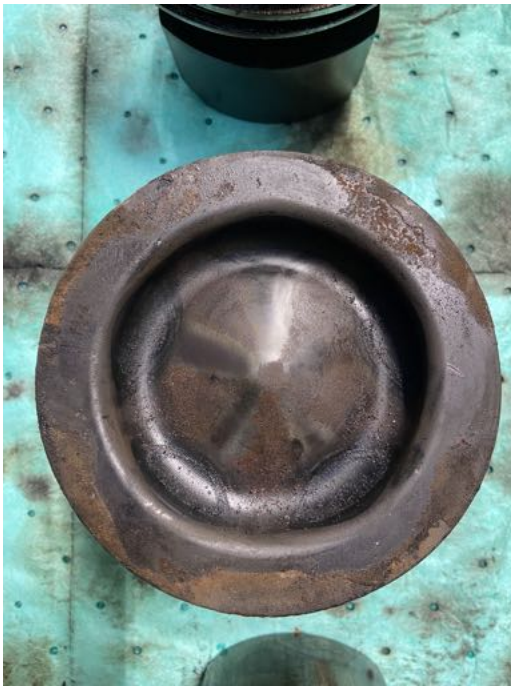
(a) Top view some visible corrosion on the bowl. Acceptable wear.
