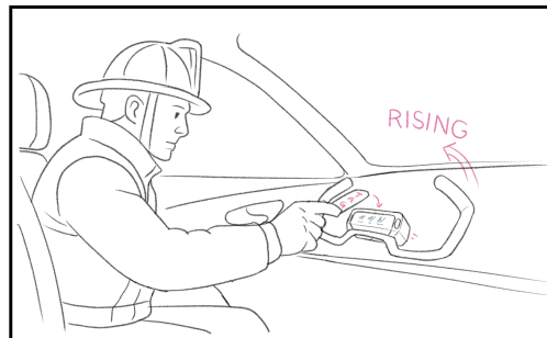
4. Firefighter taps the tag on the steering module to unlock it
