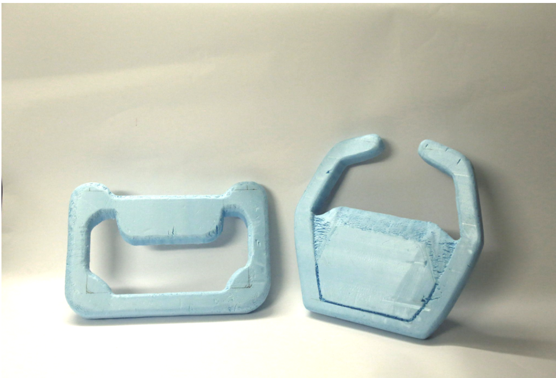
Figure 9.6: Two initial versions of the foam prototype (left with high pivot point and right with low)
