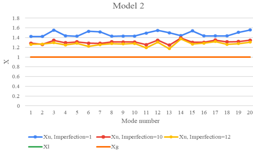
Figure 3-21 Indication of X_u extracted by FEM analysis versus calculated X_l and X_g by Eurocode equations for model-2.
