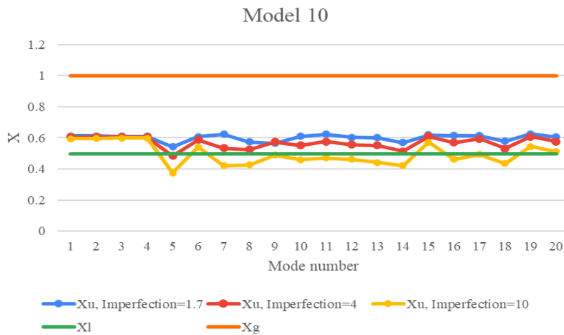
Figure 3-29 Indication of X_u extracted by FEM analysis versus calculated X_l and X_g by Eurocode equations for model-10.
