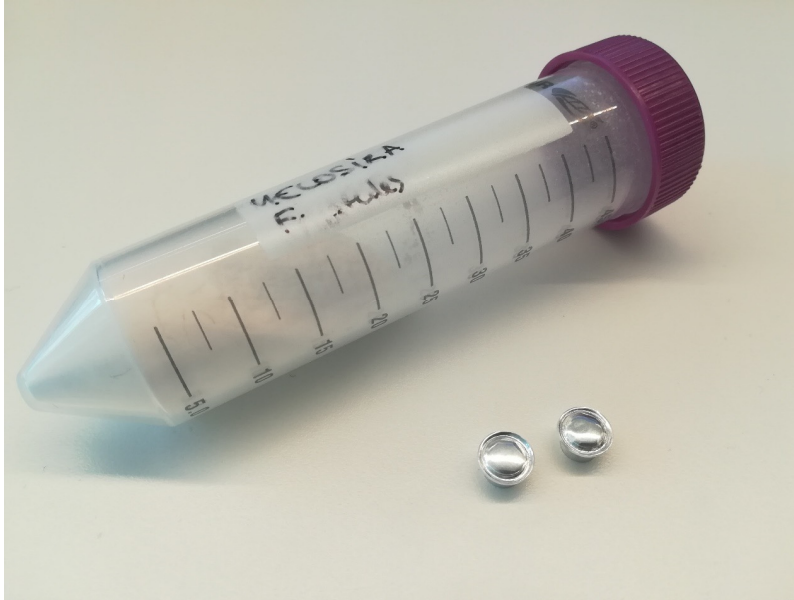
Figure 3.1 The silica powder in a plastic container and the samples for testing of specific heat capacity in small aluminum containers.
