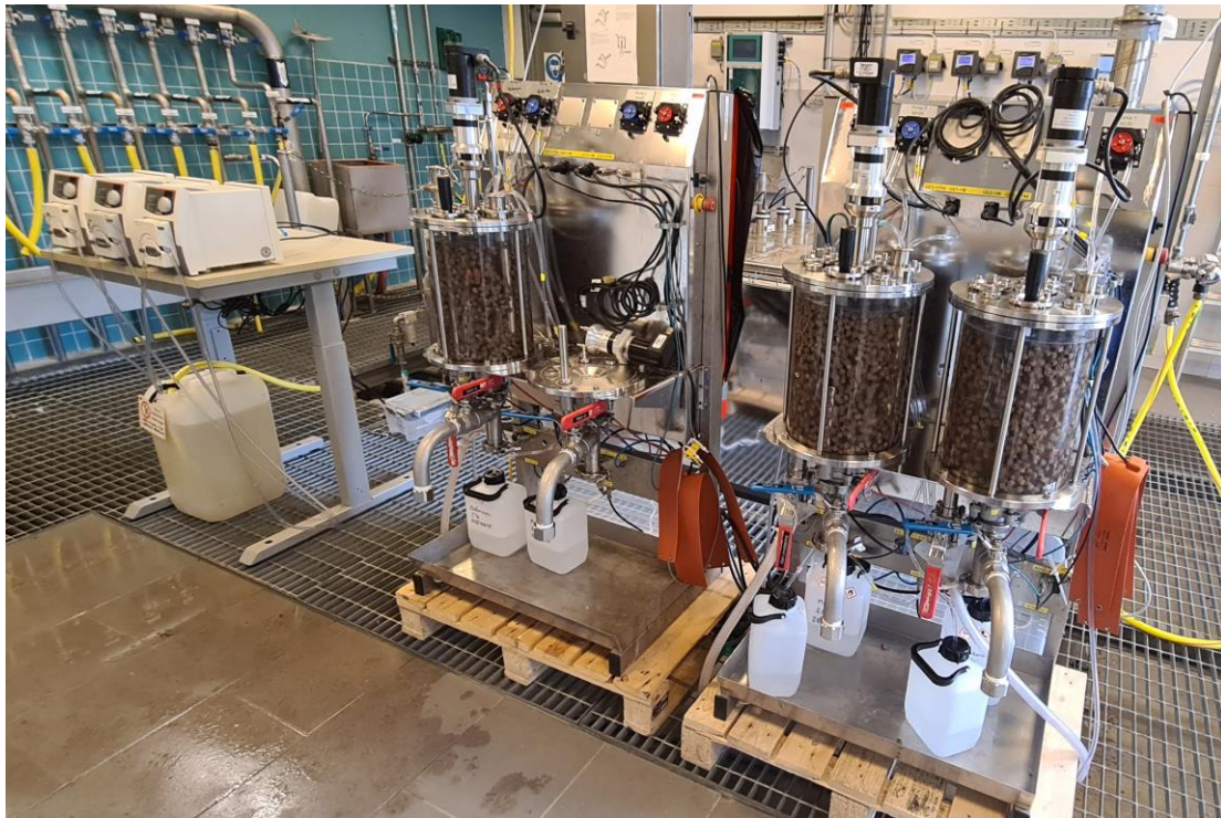
Figure 3.1. The experimental setup with reactors and influent arrangement.
