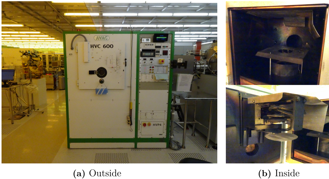
Figure 3.2: The outside and inside of the AVAC evaporator. The substrate can be mounted upside down on a holder on the inside of the door, and the source is placed in the bottom of the chamber.
