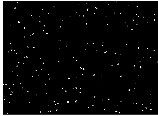
(d) \text{Ag}_3\text{Sn} particles identified after thresholding and particle analysis
