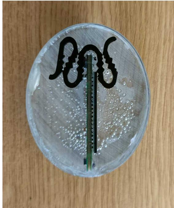
Figure 3.5: Sample cold mounted in Epoxy
