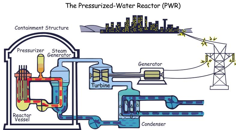
Figure 1: Schematic of a pressurized water reactor showing the two loops used to separate the water in the core from the water in the steam cycle. Source: USNRC [9]
