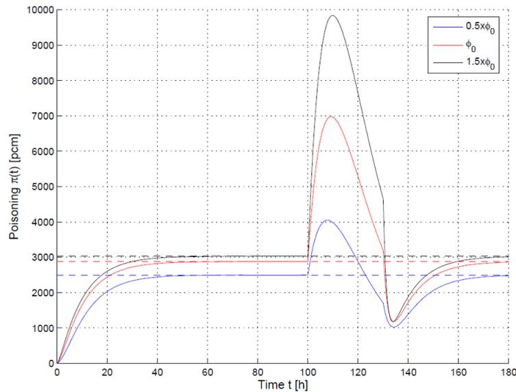
Figure 3: The decrease of xenon poisoning,  $\pi$ , which correlates linearly to the xenon concentration at different neutron fluxes,  $\phi_0$ , which correlates linearly to the power in a reactor. The reactor shuts down at  $t=100$  and is restarted at  $t=130$ . The dashed lines are the equilibrium poisonings. Picture from "Physics of Nuclear Reactors" [11].
