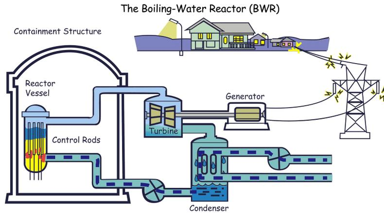
Figure 2: Schematic of a boiling water reactor showing how the water flows throughout the core, turbines and condenser etc. Source: USNRC [10]
