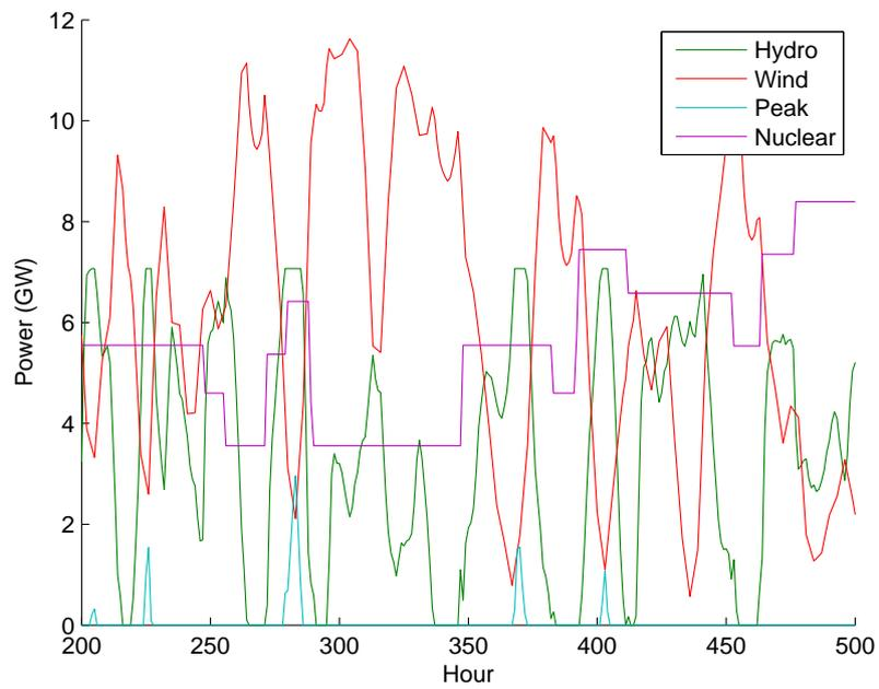
Figure 6: The middle of January with 25 TWh wind and no load following. There is some gas peak production when some reactors are shut down due to the high wind power.
