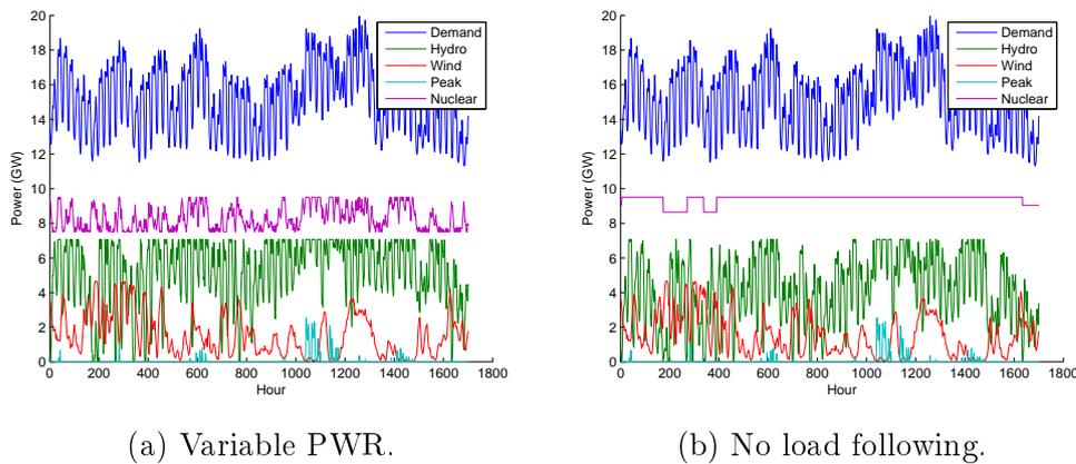
Figure 7: These figures shows the electricity system from the beginning of January to the middle of March. When load following is allowed for the PWRs, the power production becomes more variable. The figures for the whole year can be found in the appendix Figure C.1a and Figure C.3a respectively.
