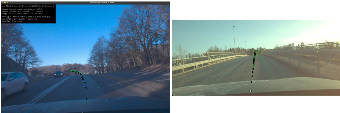
Figure 3.2: The figure shows two cases where the equipped vehicle is driving up a small hill/bridge. In both figures, some road surface condition annotations are located in the air. The motion estimation does not take vertical motion into account and could potentially cause a lot of problems as the pipeline uses these annotations to learn classification. That is, it may associate a dry road surface condition with the characteristics of trees or sky. Image by author.
