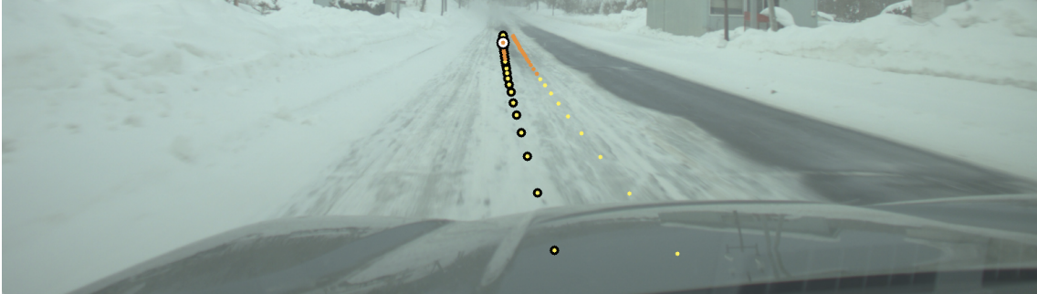
Figure 3.1: A part of an example image in the dataset that will be used in the project. Note that the image is cropped so that it only shows the road with annotations. The conditions with the highest probability in the point-wise road surface condition estimations are annotated as coloured circles in the image. The yellow and orange colours correspond to the road surface conditions of snow and grey ice. Image by author.
