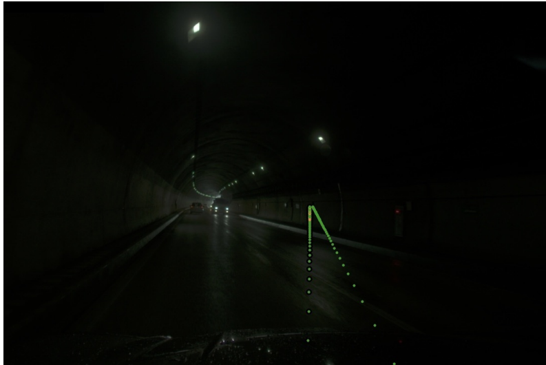
Figure 3.5: The figure showcases a scenario where the recording vehicle is driving under a tunnel. The estimations used to create laser annotations are based on GPS data, and the tunnel severely limits the ability to receive such data. Consequently, this results in laser annotations incorrectly placed outside the recording vehicle’s driving path. Image by author.
