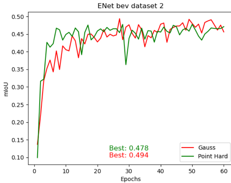
Figure 4.37: mIoU graph for bev data on the second dataset trained with ENet model.
