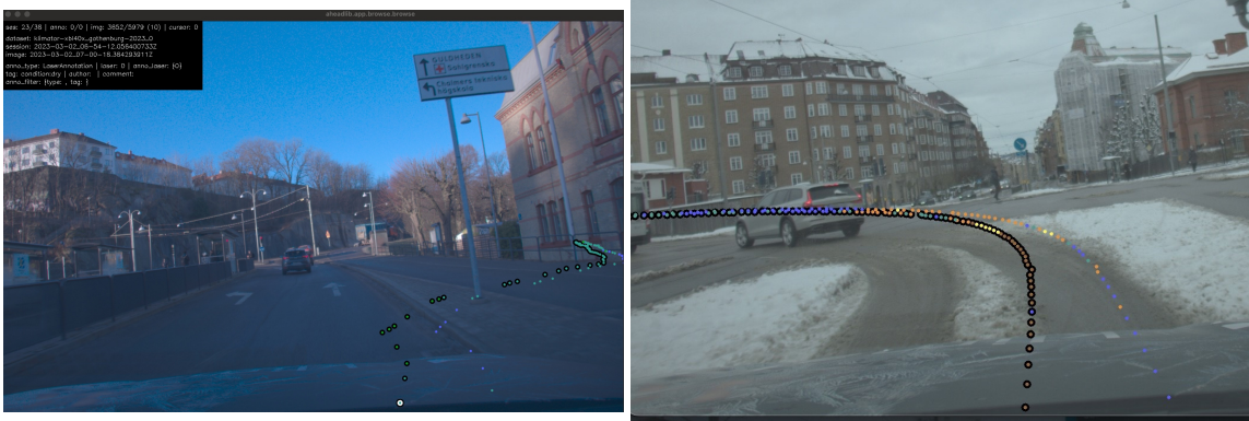
Figure 3.3: The figure shows annotation problems while the vehicle is turning. In the left figure, the vehicle is driving in an urban landscape, which includes a lot of smaller turns. The motion estimation utilises the vehicle’s yaw rate. Therefore, smaller turns with a temporarily big yaw rate will cause the motion estimation to assume a large change of direction. As seen in the figure, situations like these can cause the annotations to be completely off the vehicle’s actual path. In the right figure, the vehicle is performing a larger turn. The annotations close to the vehicle are reasonable, but the annotation method still struggles to locate the annotations further away. Image by author.
