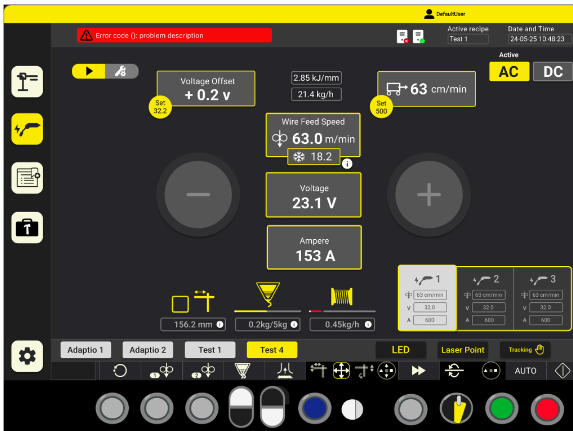
Figure 49: Feedback with clear error codes and alerts. Interactive info texts to help operators diagnose and resolve issues effectively. Visual alerts for the HMI in critical situations.
