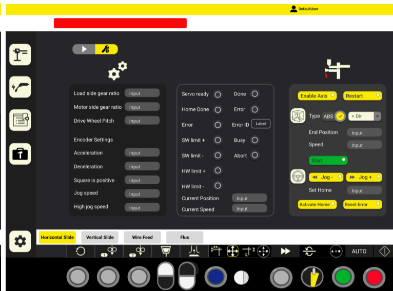
Figure 10: Welding parameters settings view iteration one.
