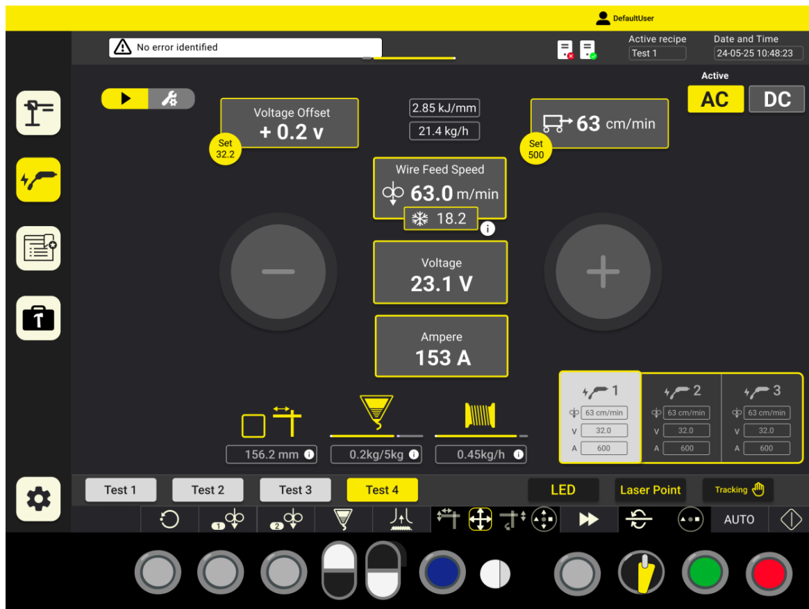
Figure 45: Displaying relevant information of critical parameters such as voltage, current, and speed in logical views to help operators understand the current state of the system.
