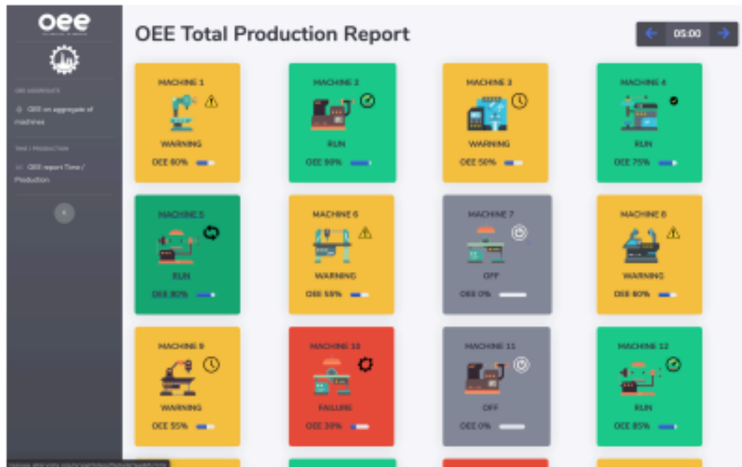
Figure 5: Andon interface separating graphics (Di Gregorio et.al., 2020)
