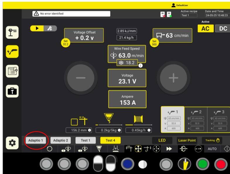
Figure 42: Recipe added to bottom bar of main welding view
