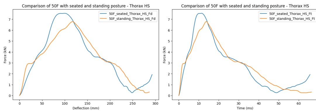
Figure 59 - Comparison of seated and standing position of 50F - force-deflection and force-time plot at 9.5 m/s impact speed on thorax.
