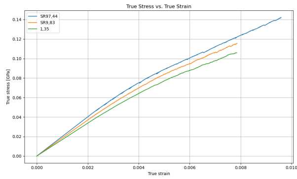
Figure F.1: Stress-strain curve for a dogbone specimen modeled using the Male 50 material card.
