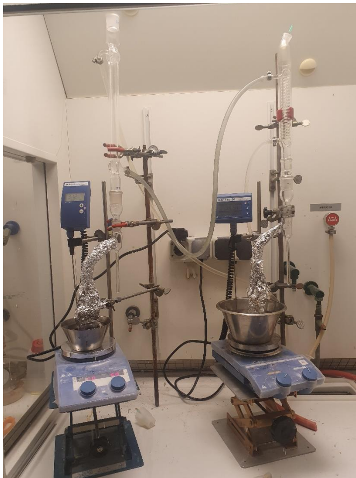
Figure 9. The set-up for the factor trial with Dean-Stark apparatus.
