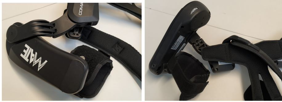
Figure 2.13: Torque generator box and arm cuff of the Mate exoskeleton
