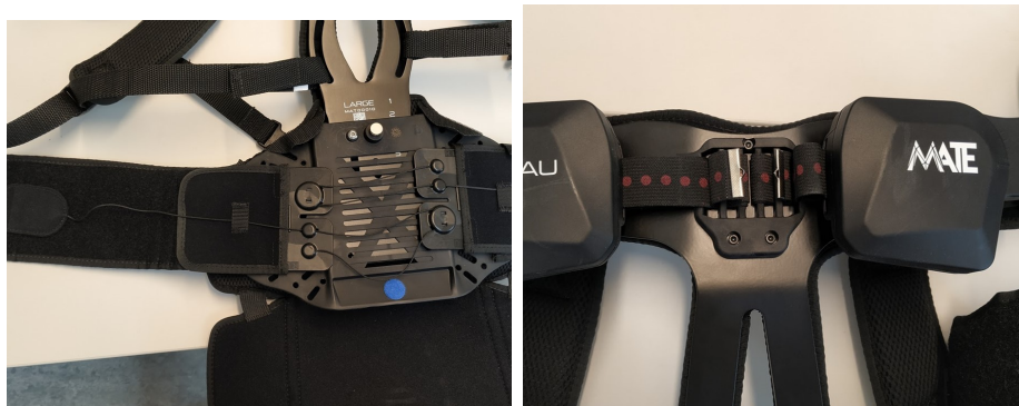
Figure 2.12: Belt, back and shoulder adjustments on the Mate exoskeleton
