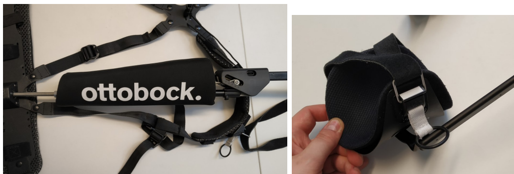
Figure 2.5: Cable pull technology and arm cuff of the Paexo exoskeleton
