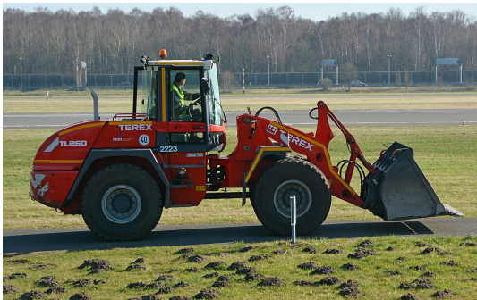
(a) A wheel loader with an articulation joint, shown from the side.
