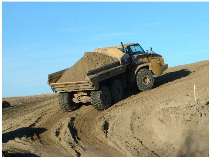
Figure 2.1: An example of an articulated vehicle, a Caterpillar 740 Ejector articulated haul truck driving up a hill [2].
