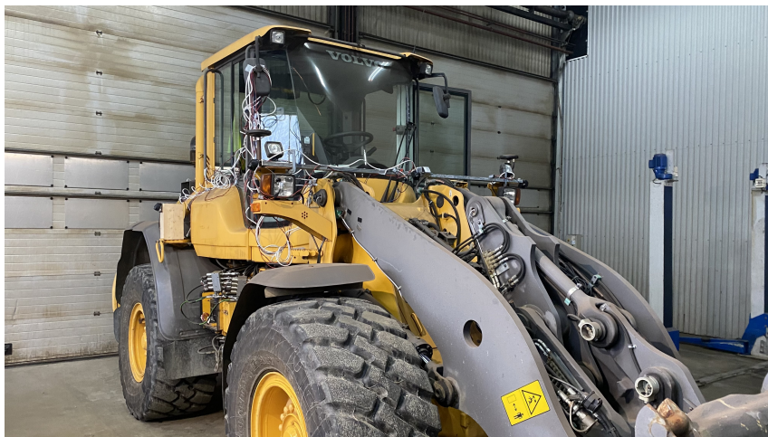
Figure 3.9: The wheel loader used for real-world data gathering and testing with mounted cameras and IMUs.
