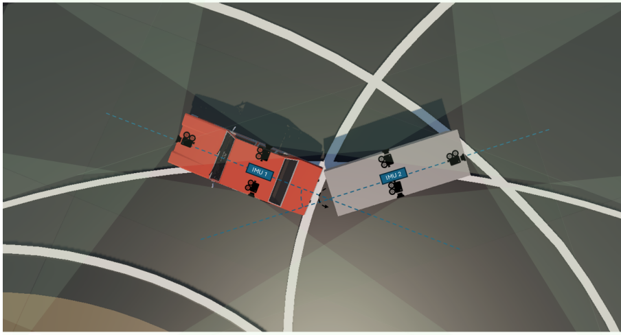
Figure 1.2: Sensor setup of the 2-body vehicle, the basis of this project.
