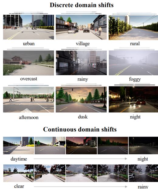
Figure 1.1: Common examples of domain shift in autonomous driving [6]. Variations in architectural styles, weather conditions, and lighting are typical scenarios where domain shift occurs.
