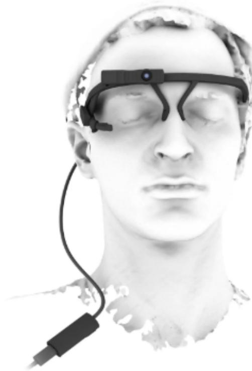
**Figure 3.2:** Headset configuration used for gaze tracking [2]
