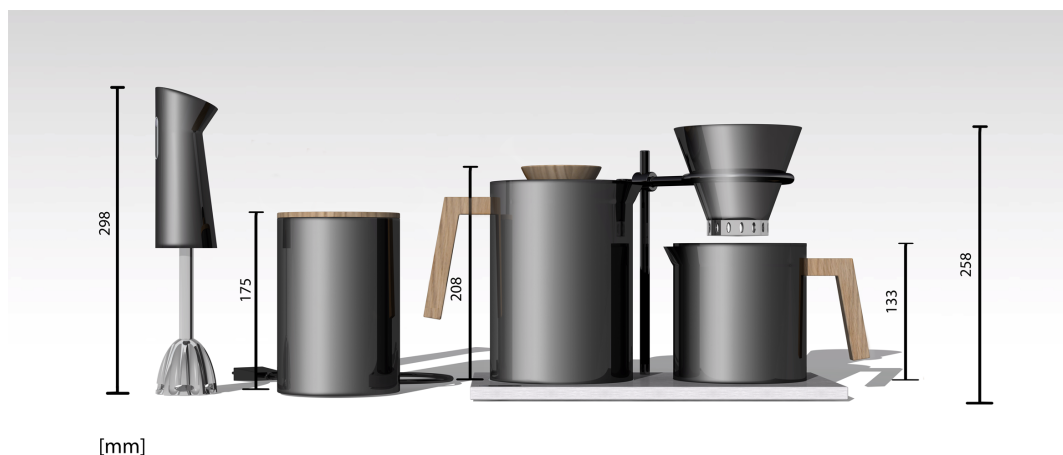
Figure 6.11: Measurement of the final concept. Author's own copyright.
