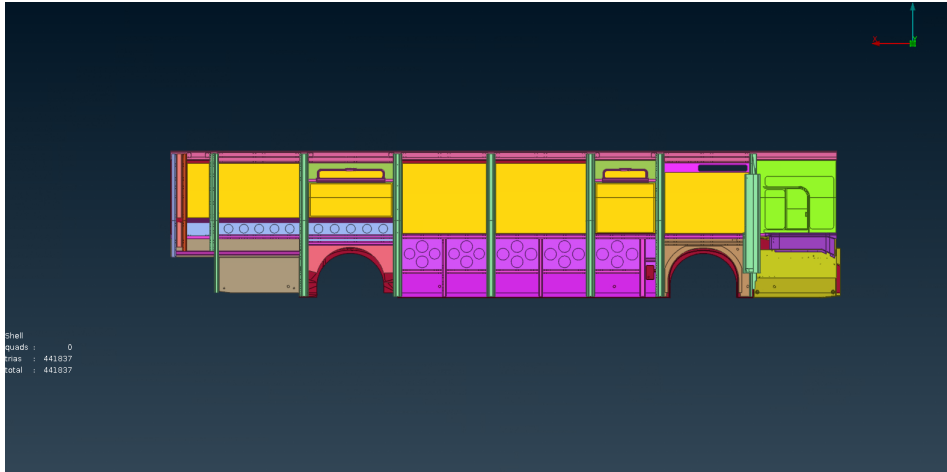
Figure 3.10: Modified left-hand wall
