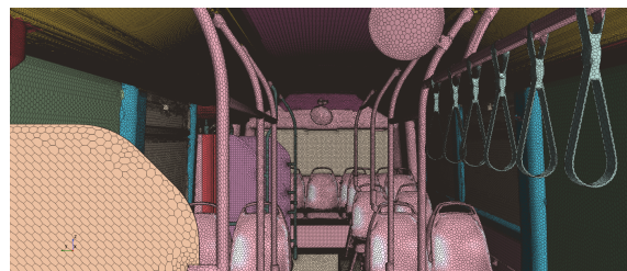
Figure 3.4: Surface Wrap of the Interior of the Bus
