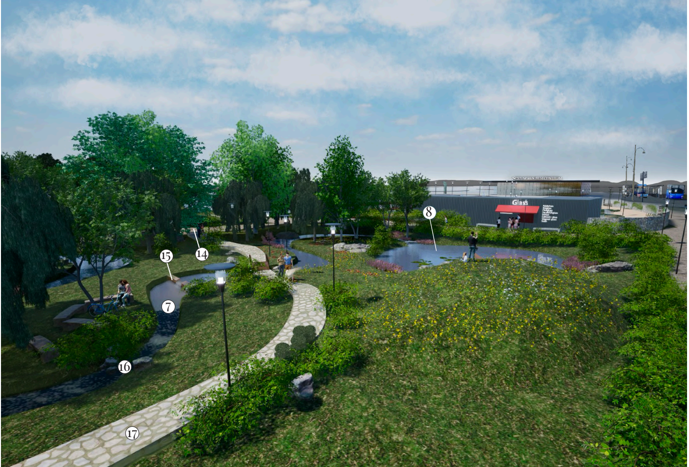
Figure 3.22. This perspective highlights the stormwater system, where water first enters the forebay, then passes through the gabion before reaching the ditch. In the background, the gelateria can be seen in front of the golf course and Stenpiren Resecentrum, linking the new landscape to the urban context.
