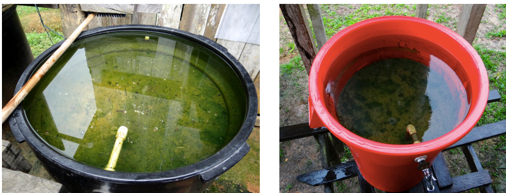
Picture 4.2. Two-step systems with visible schmutzdecke.
