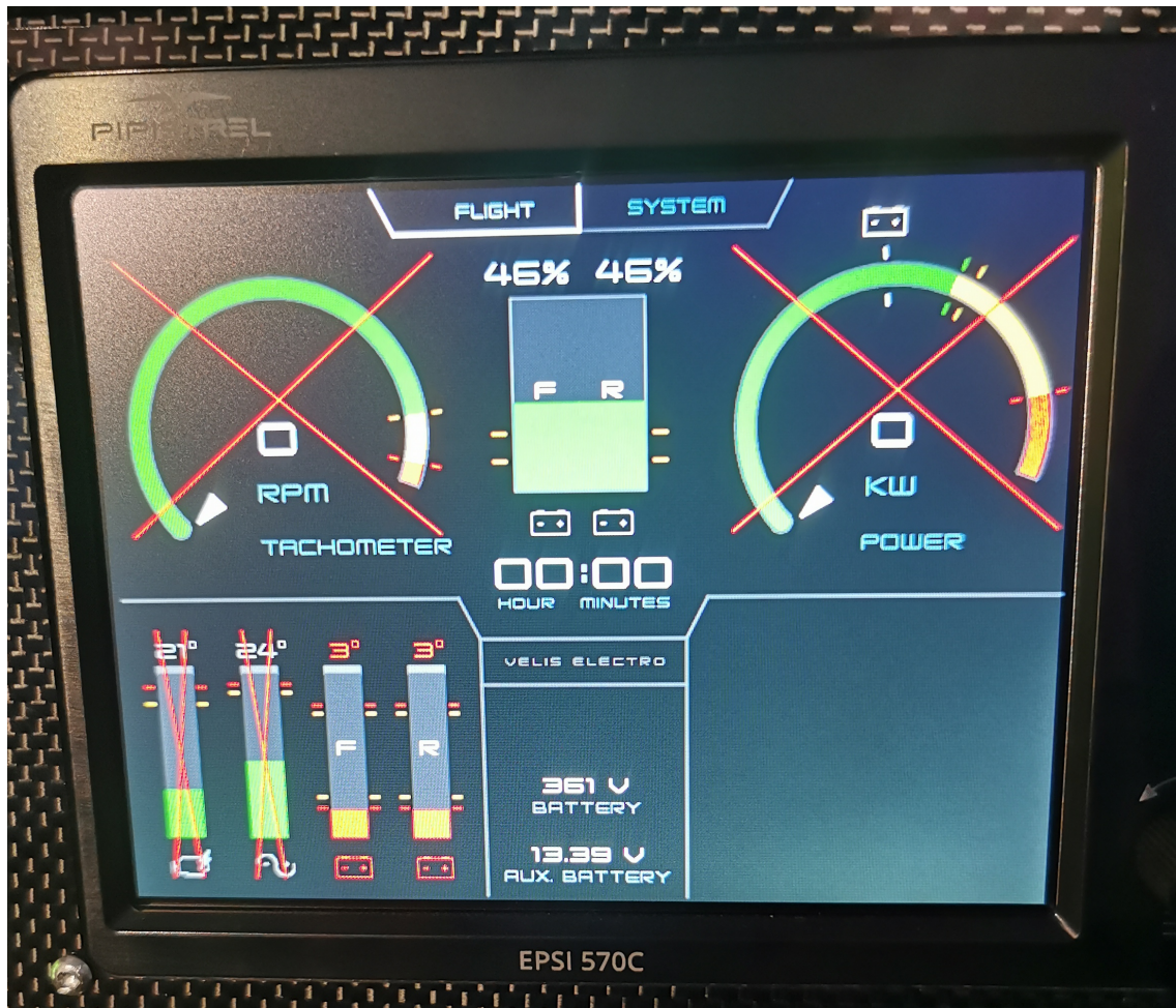
Figure 4.1: Picture of a battery HMI taken during the field study
