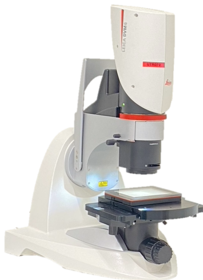
Figure 3.4: Picture taken of the light microscope where the transmitted light insert on can be seen attached on the stage.
