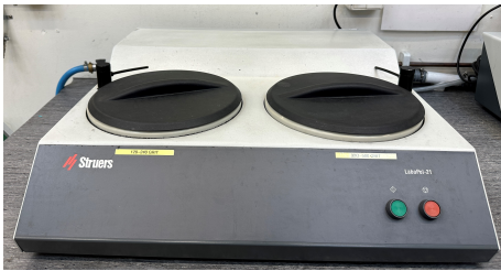
(a) Struers labopol-21 for chamfering the edge
