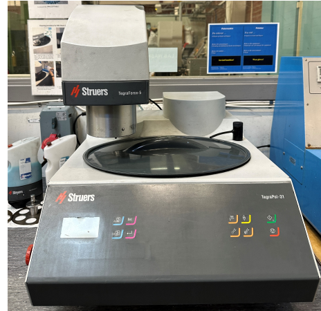
(b) Struers Tegrapol-31 for grinding and polishing
