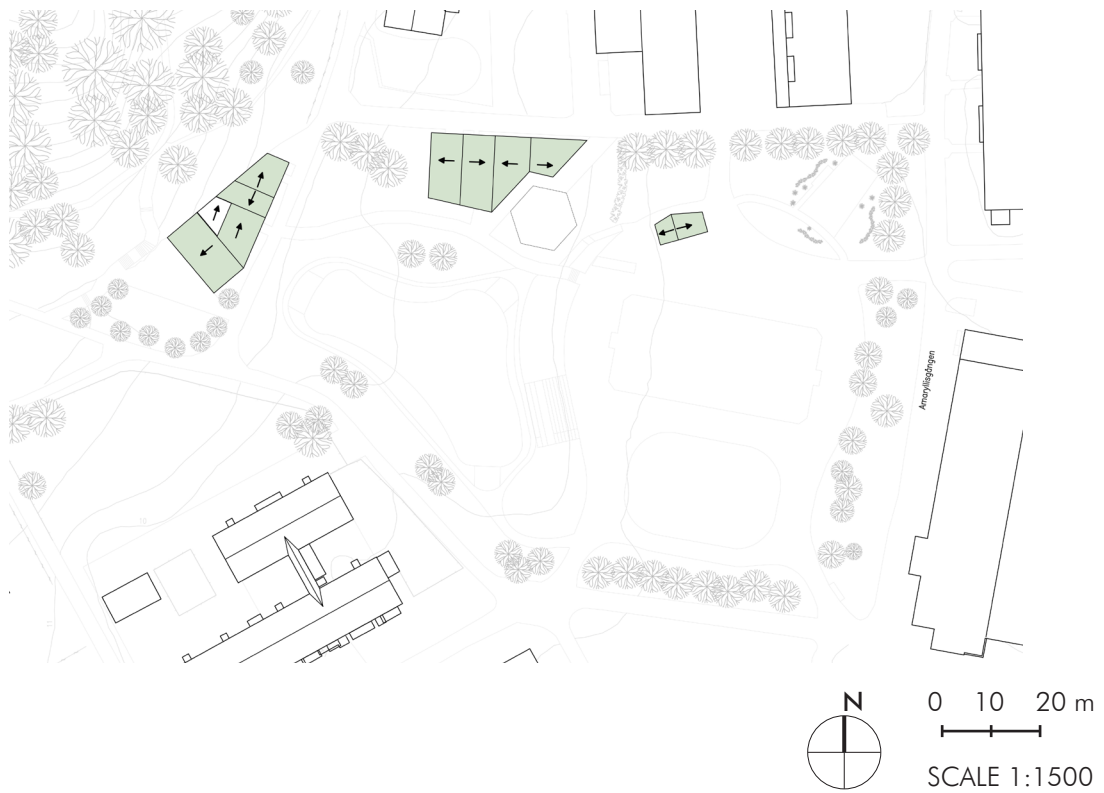
Top view of the roofs showing direction of the slope on the new buildings.
