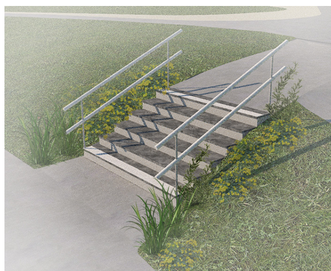
Model of the stairs. The top material is dark natural stone with texture for anti-slip effect. The bottom and top steps are marked with white for clarity.
