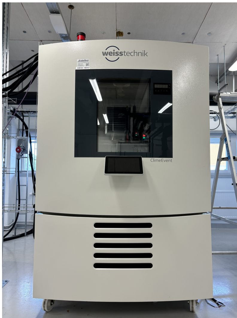
Figure 4.3: Weiss Technik Reach-In Battery Test Thermal Chamber
